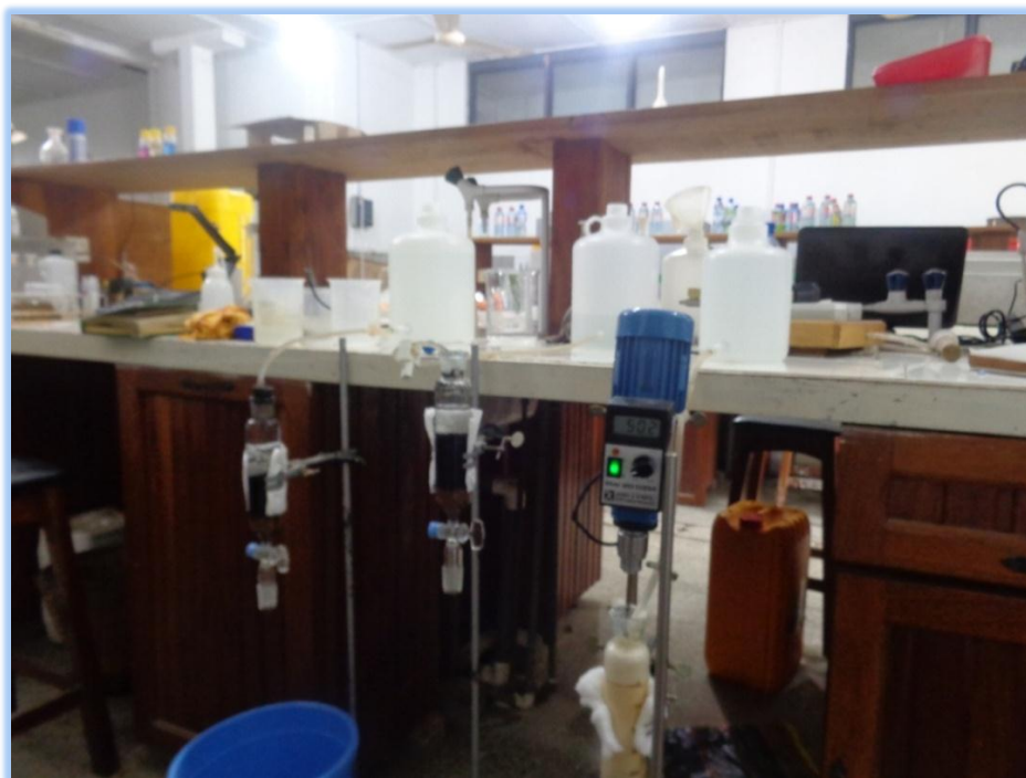
Plate 3-5a Adsorption Column set ups for AOCC
