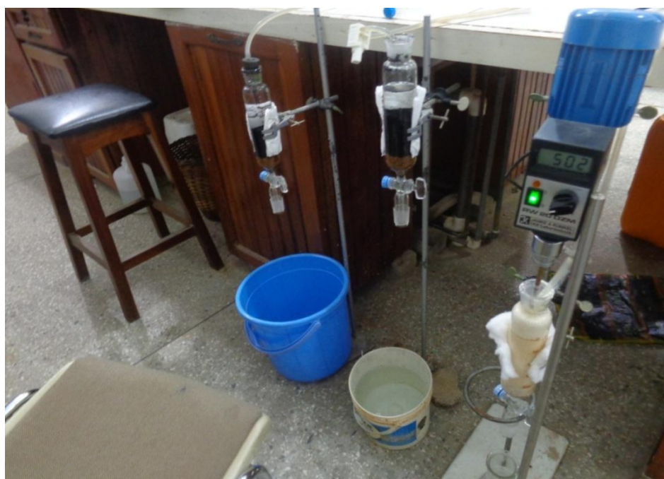
Plate 3-5b Adsorption Column set ups for AOCC
