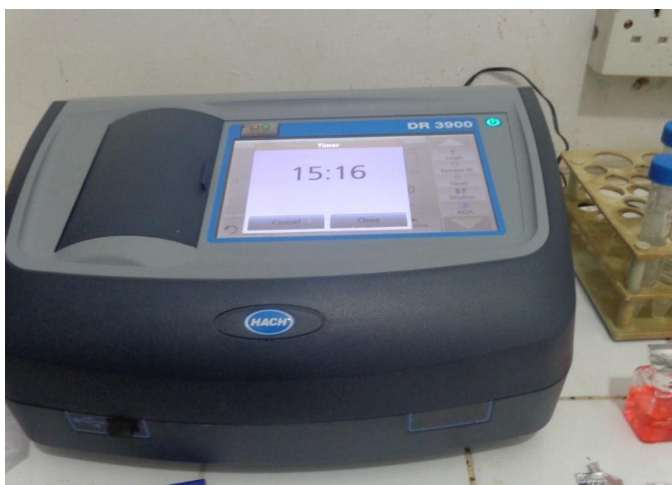
Plate 3-7. Hach Spectrophotometer used in Contaminant Concentration Measurements
