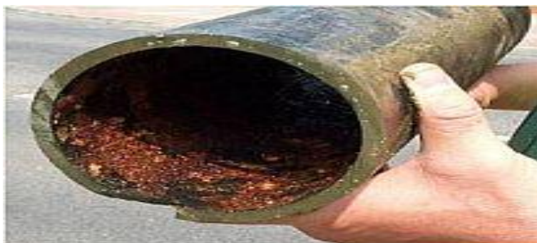
Plate 1: Biofilm growth inside a pipe (Source: Raju et al. , 2010)
