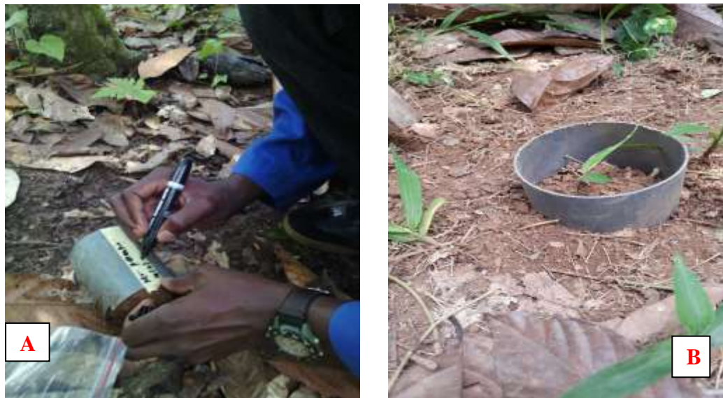
Plate 3.2. The use of PVC core sampler. A) PVC sample being buried into the soil to a height of 10 cm. B) Labelling the PVC sampler containing the soil
