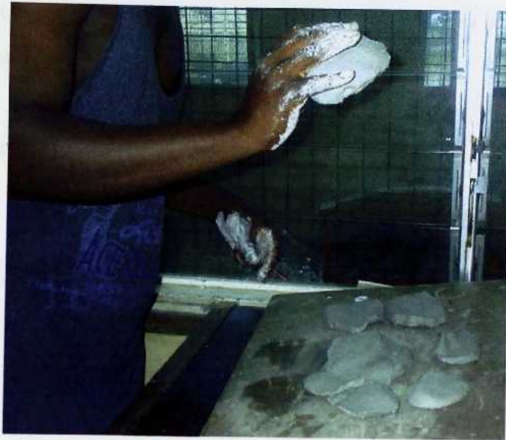
Plate 11 Banging the clay slices on each other
