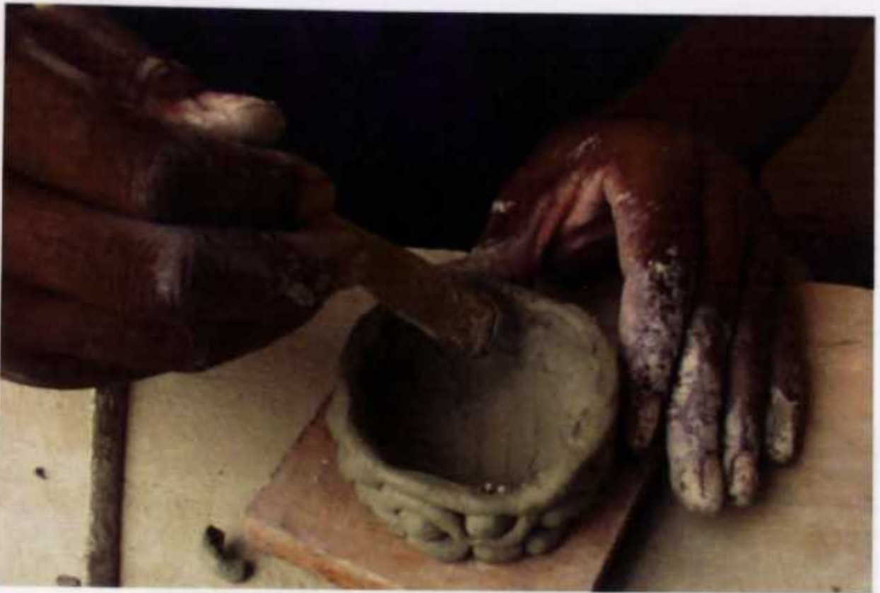
Plate 63 Smoothing inside the pot made by joining the various techniques
