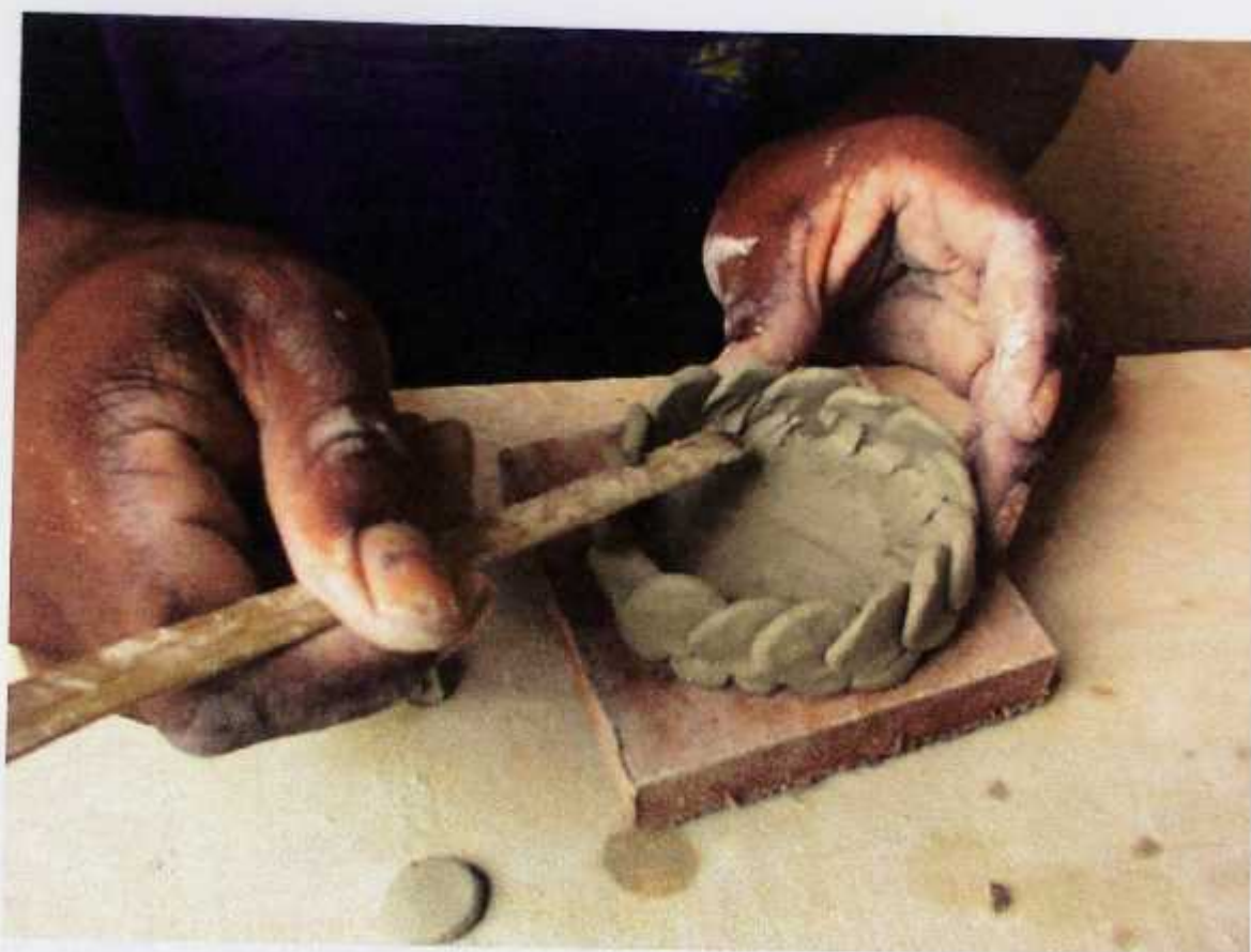
Plate 54 Joining the clay buttons to the base
