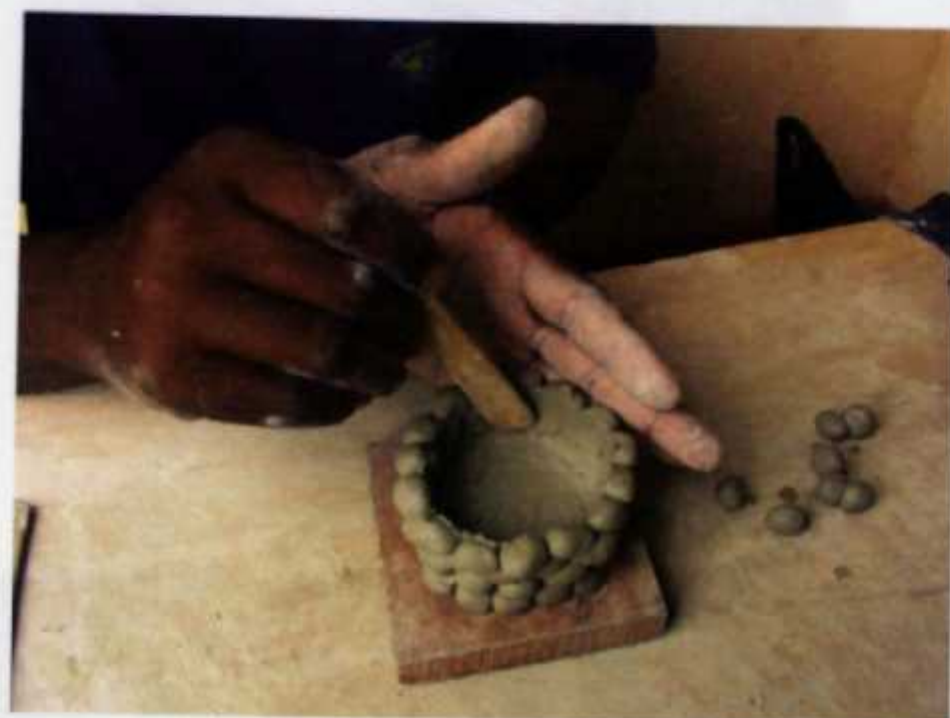
Plate 38 Smoothing inside the wall of the clay ball pot
