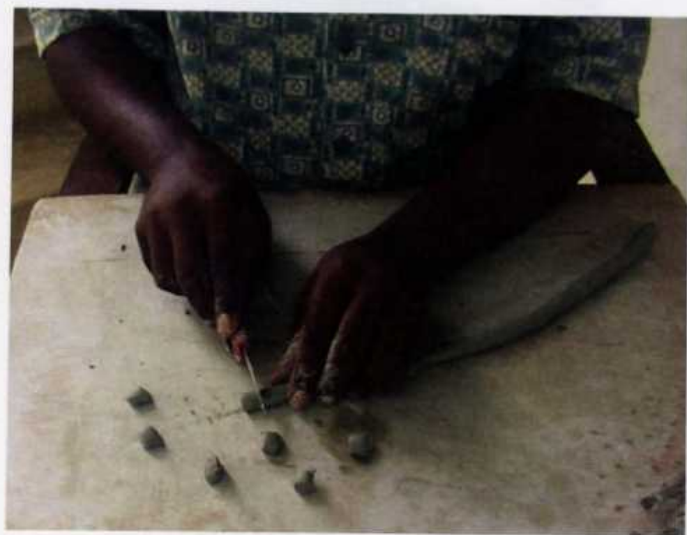
Plate 29 cutting the coil with knife
