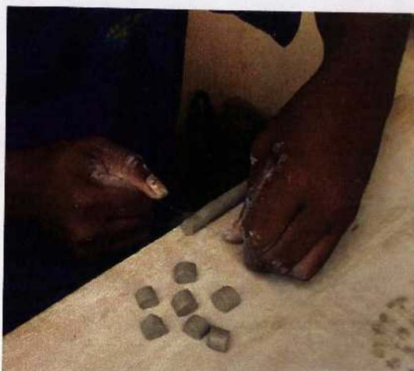
Plate 57 Cutting the short coils using cutting wire
