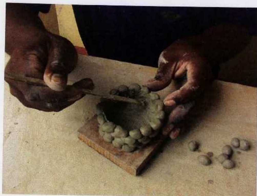
Plate 37 Raising the wall of the ball pot by joining the clay balls
