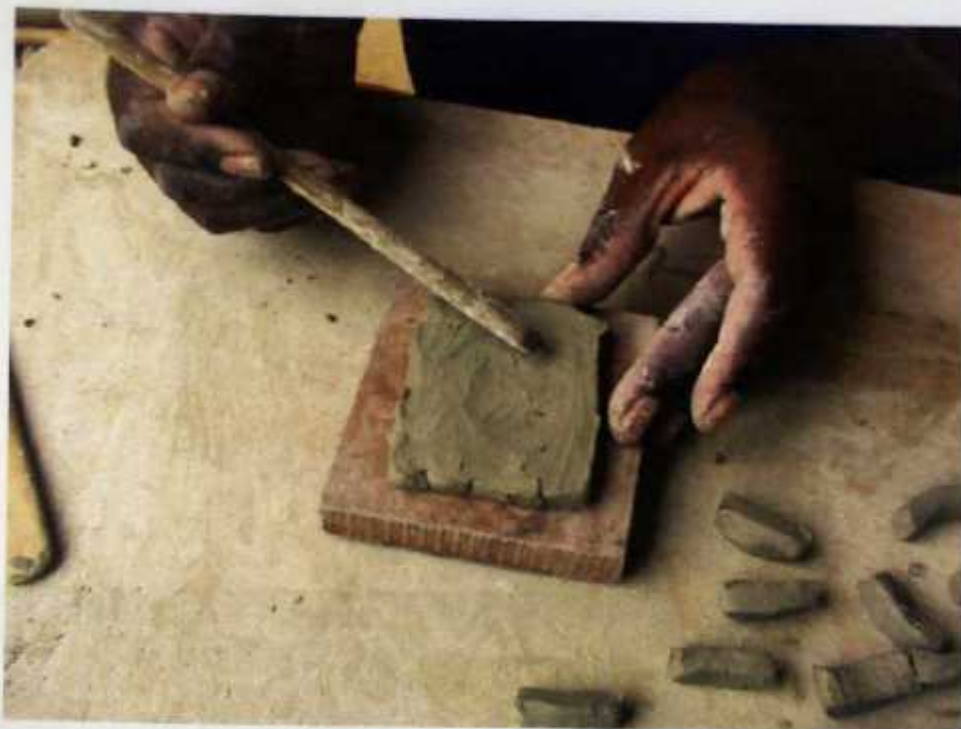
Plate 67 Joining bricks at the base
