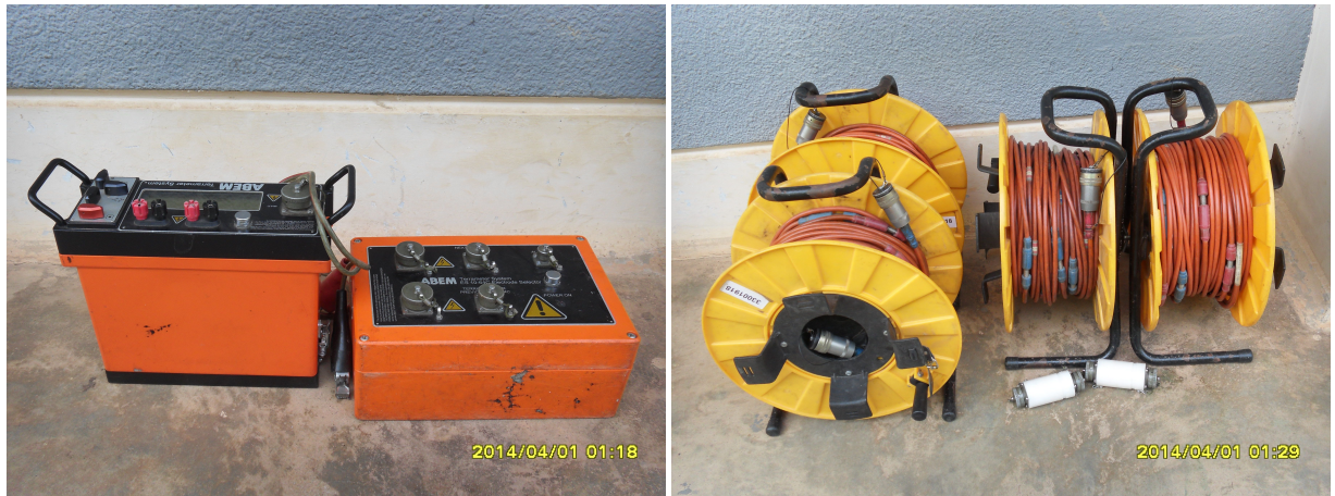
Figure 3.5: The ABEM Terrameter SAS 4000 device, electrode selector ES 10-64C and multi-core cables with their connectors.
