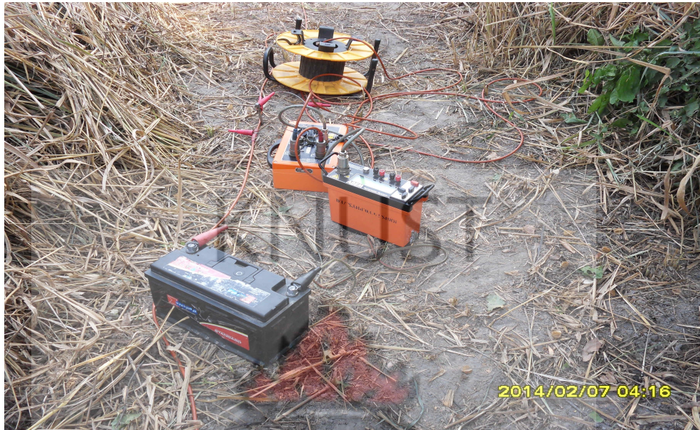
Figure 3.6: A setup of the ABEM Terrameter taking readings.
