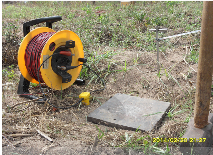
Figure 3.11: Picture of a trigger geophone connecting the trigger cable beside a metal block at the shotpoint.
