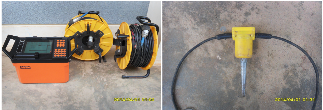
Figure 3.9: Pictures of the Terraloc Mark 6, refraction seismic cables and spiky 10 Hz geophone.
