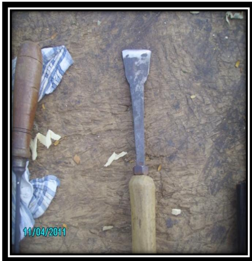
Plate 4.21a Locally manufactured chisel
