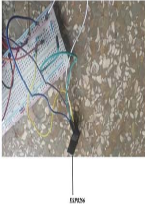
Figure 7: Installation of the ESP8266 Module
