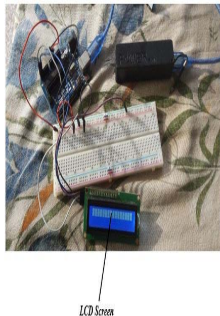
Figure 4: Installation of Arduino Uno and LCD
