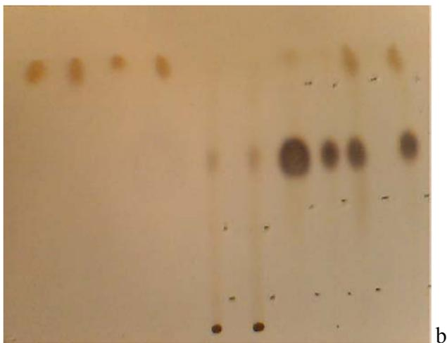
**Figure 3.18 TLC Chromatograms for ether, chloroform, water, ethanol and methanol extracts of Griffonia seeds a) under 254nm b)white light**
