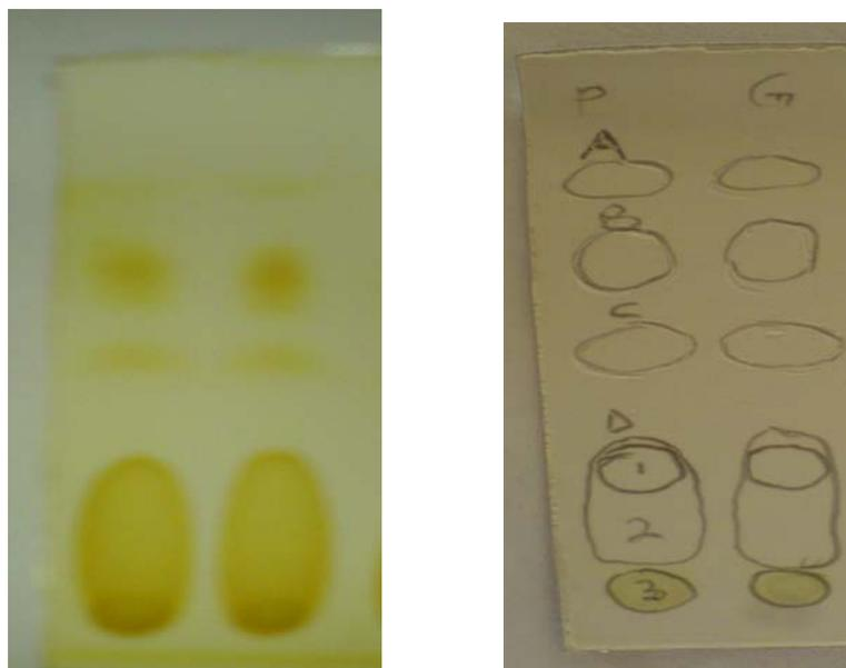
**Figure 3.20** TLC chromatogram for pet ether extract using pet ether/chloroform 50:50 as mobile phase and silica as stationary phase and iodine vapour as detecting reagent
