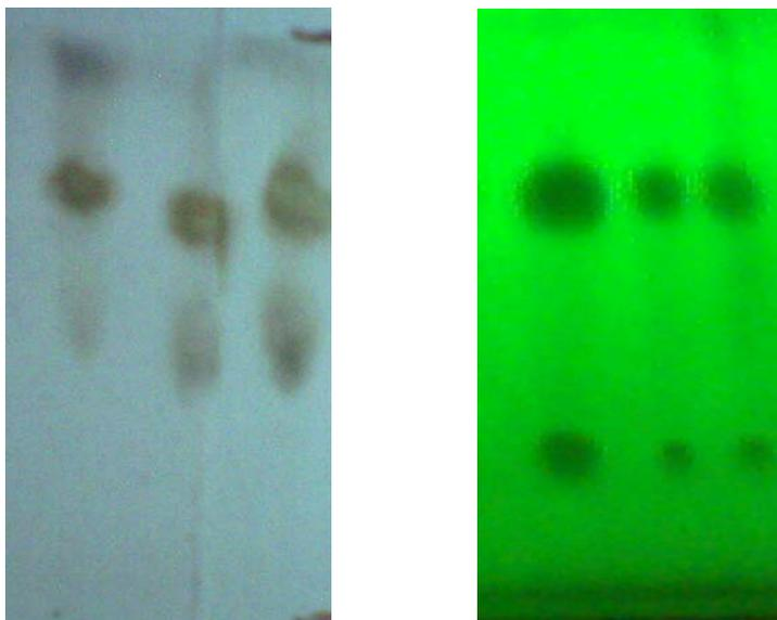
**Figure 3.19** TLC chromatogram of aqueous methanolic extract of seeds of 5-HTP using butanol:water:acetic acid 12:5:3 as mobile phase. a)after spraying with 5:95 H<sub>2</sub>SO<sub>4</sub> in methanol b)under 254nm
