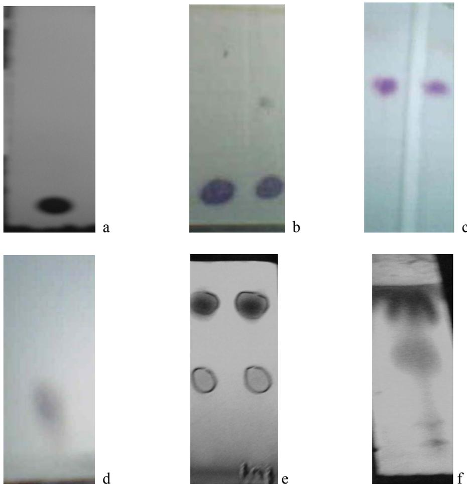
Figure 3.16 Chromatograms showing separations offered by various solvent compositions on a silica stationary phase a)  $\text{CHCl}_3$  b) 5:95 methanol in  $\text{CHCl}_3$  c) 20:80 methanol in  $\text{CHCl}_3$  d) 20:80 ethanol in Chloroform e) n-propanol : water:acetic acid 12:5:3 f) ethanol : water :acetic acid 12:5:3
