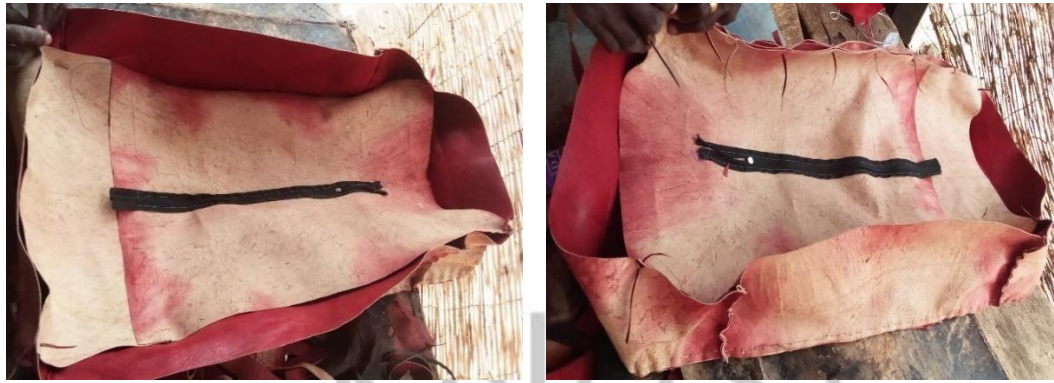
(a) Fixing of Zipper (b) Holding the Edges in Position with Stitching Pins
