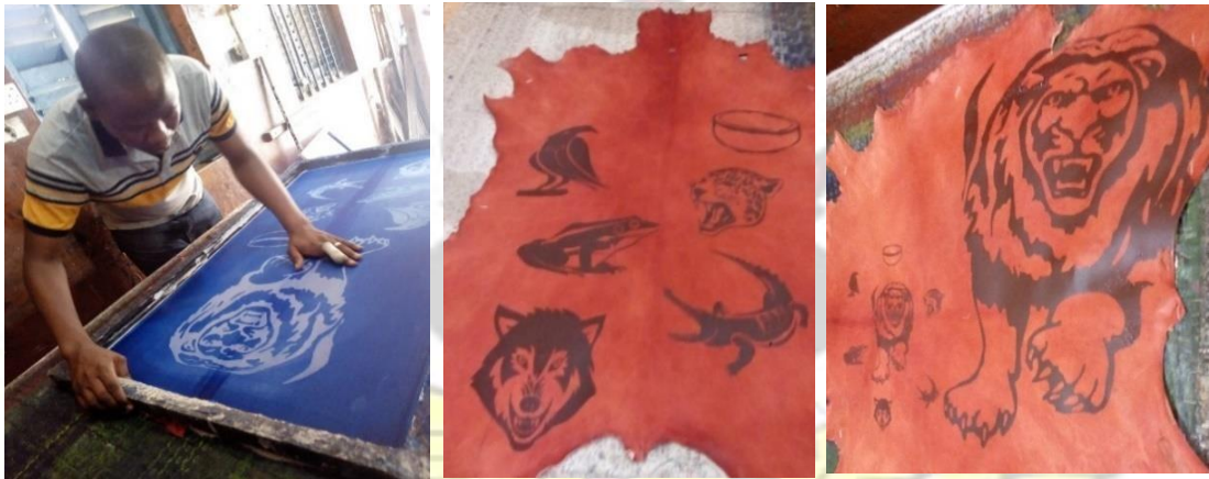
(a) Researcher Setting Screen (b) Printed Totems (c) Printed Lion
