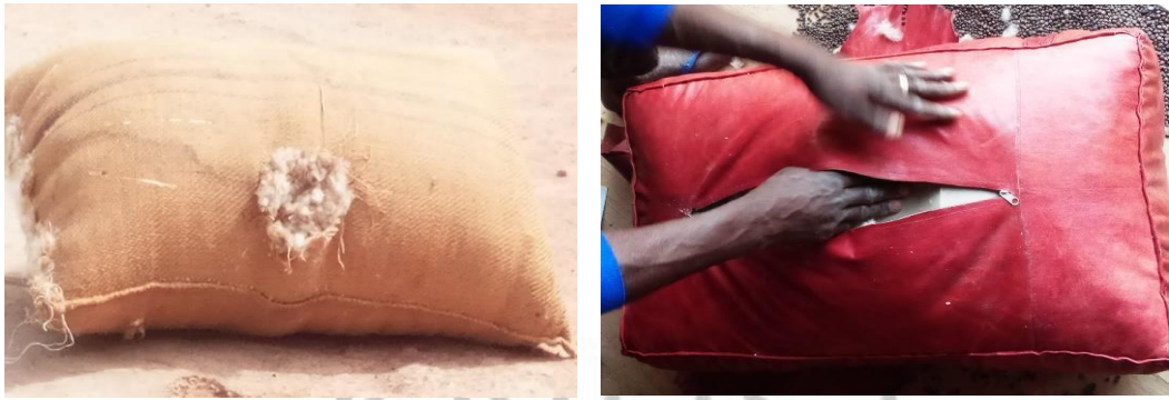
(a) Bag of Kapok Fibres (b) Filling of Bottom Rest Cover with Kapok Fibres
