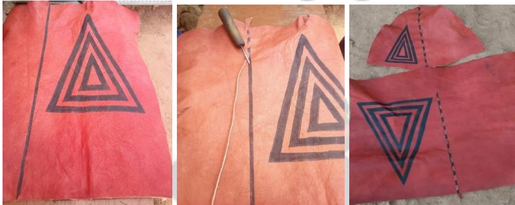
(a) Line on the Shaft (b) Creating Running Stitch (c) Finished Running Stich Plate
