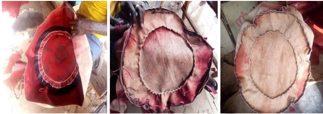
(a) Joining Side Strip to Top (b) Fastening the Together (c) Sticking
