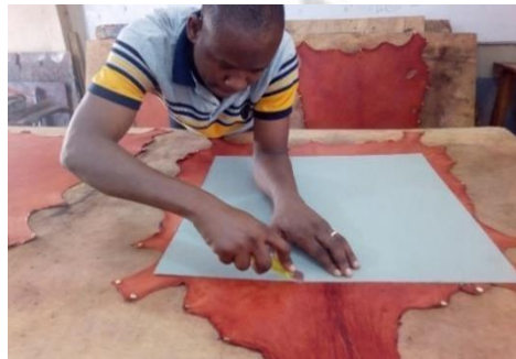
Plate 3.13: Researcher Cutting Template Shape on Leather (Source: Studio Work, 2020)
