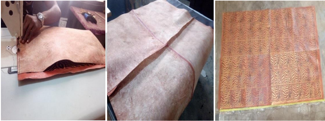
(a) Stitching of Printed Leather (b) Application of Glue (c) Joint Leather Pair
