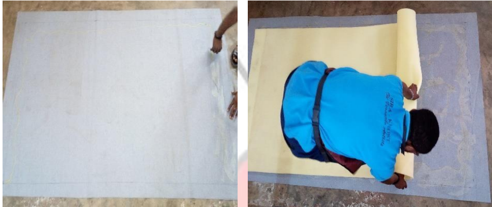
(a) Marking on Leatherette (b) Bonding of Foam & Leatherette
