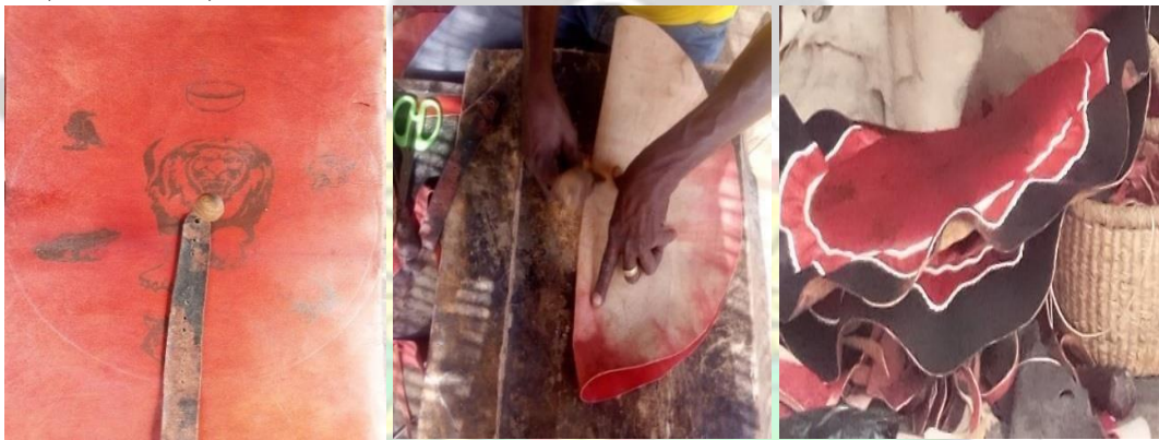
(a) Measuring Belt (b) Creating Central Point (c) Fixing White-leather on Edges
