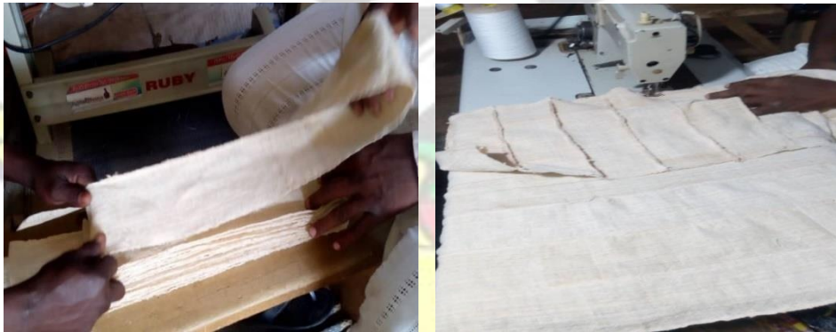
(a) Measuring Woven Strips of Smock (b) Joining of Woven Strips of Smocks
