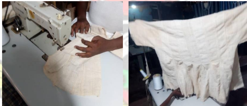
(a) Sewing of Sleeves (b) Sewn Sleeves
