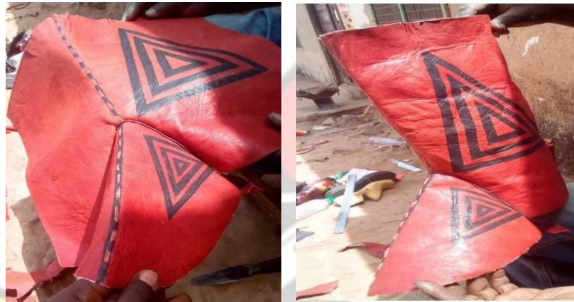
(a) Joining Instep to the Shaft (b) Closed-up Shaft
