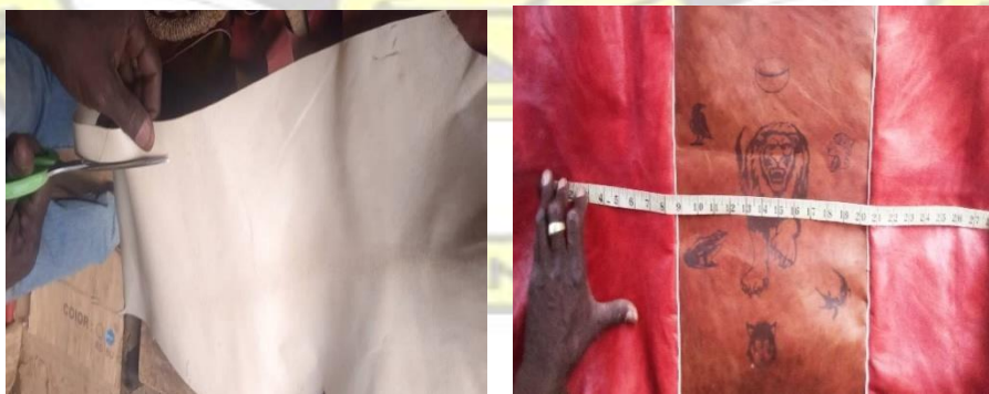
(a) Cutting of Leather Strip (b) Demarcated Segments with Strips Plate
