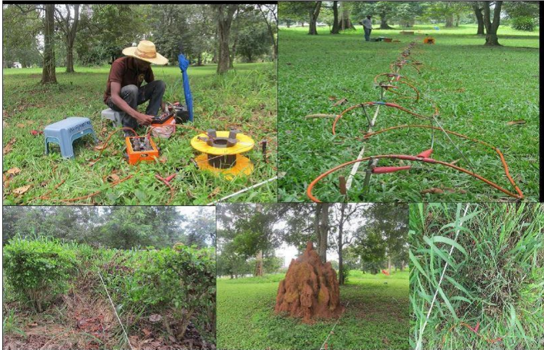
Figure 3.6: Data acquisition with the ABEM Terrameter on different profiles
