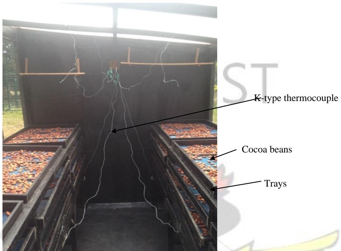
Fig 3.7b: Display of temperature measuring connectors
