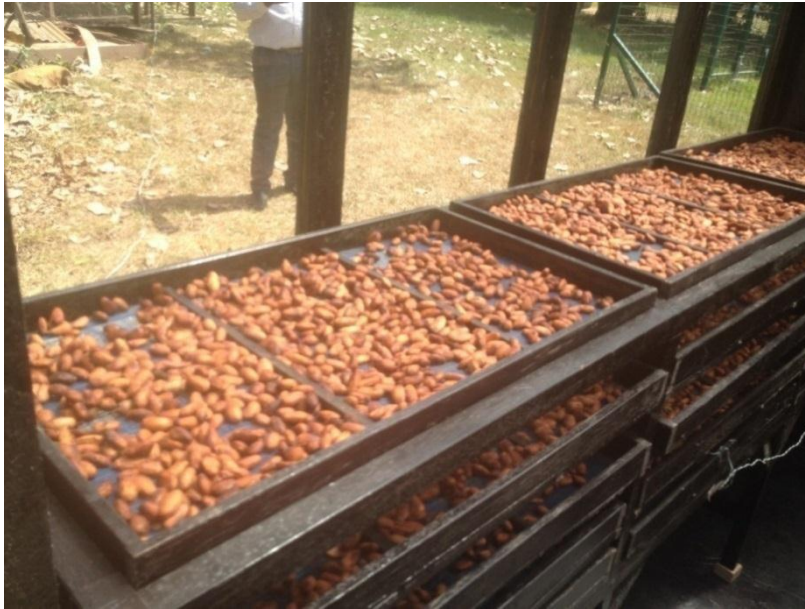
Fig 3.2b: Arrangement of cocoa beans inside solar dryer
