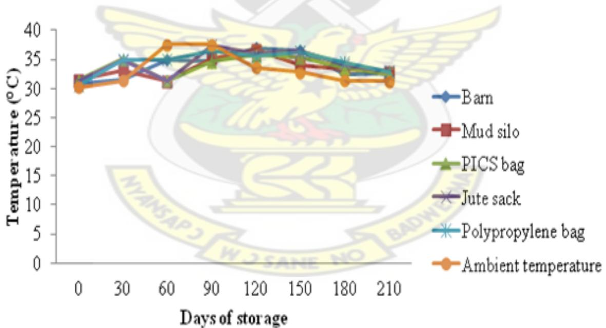
Figure 26: Relationship between ambient temperature and among internal temperatures of storage structures
