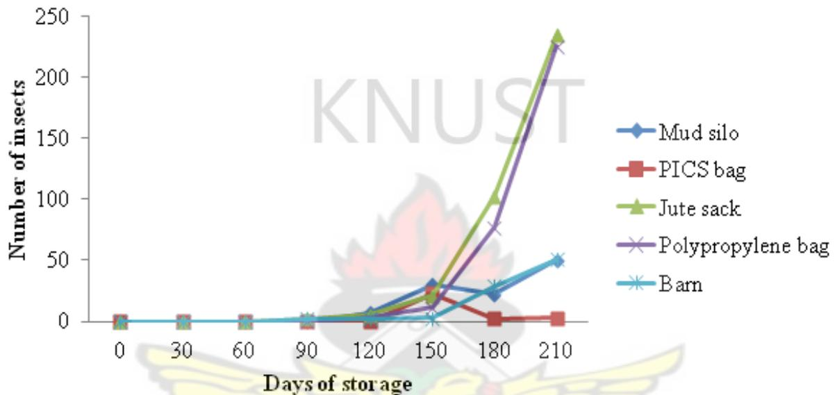
Figure 32: Live insects counted from 1 kg samples of the sorghum grain stored in the various storage structures
