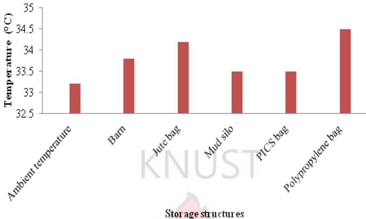
Figure 27: Mean temperatures of various storage structures
