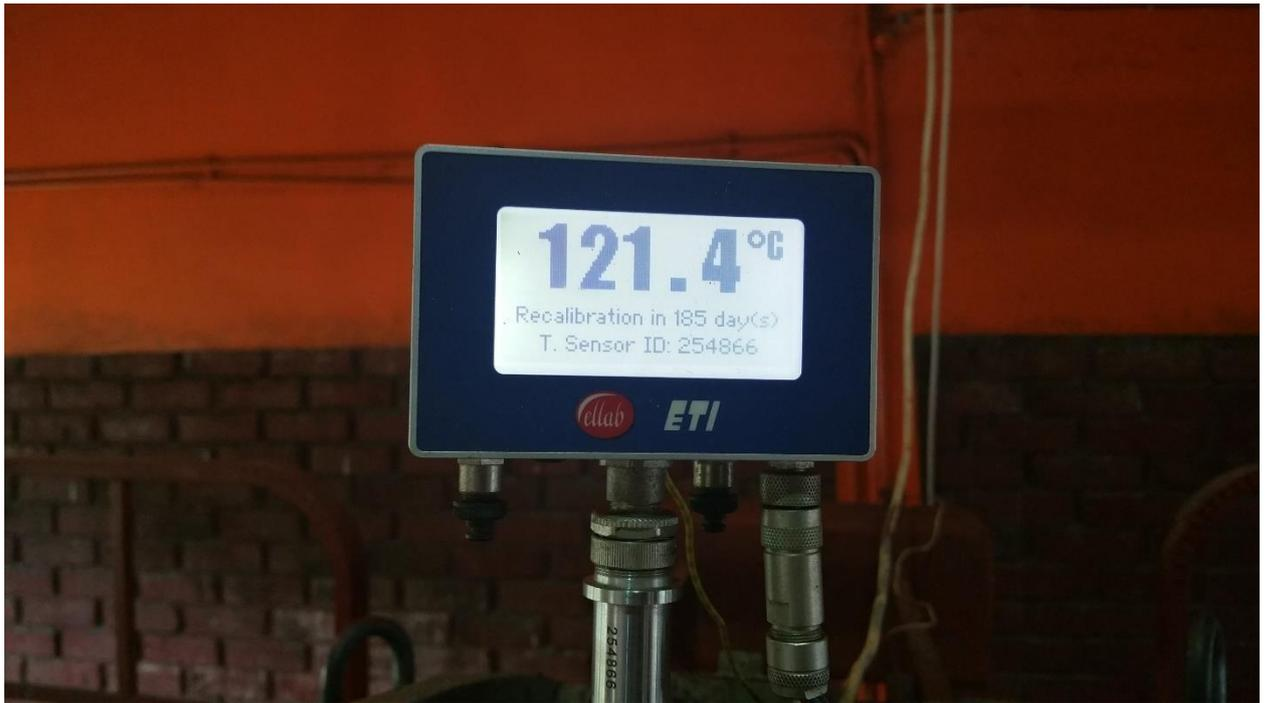
**Plate 15: Ellab Temperature Indicator (Reference Temperature Indicator) device showing autoclave temperature readings.**
