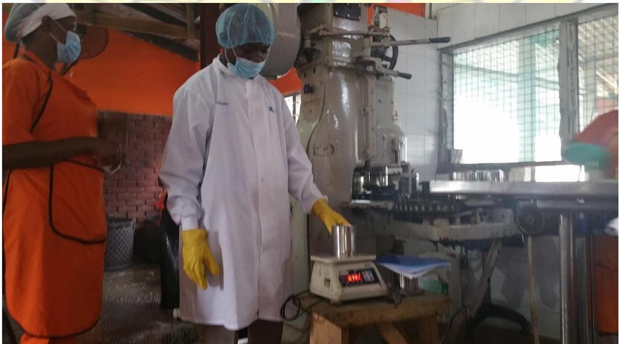
**Plate 12: Author checking the weight of the seamed product to ensure specified net weight is met.**
