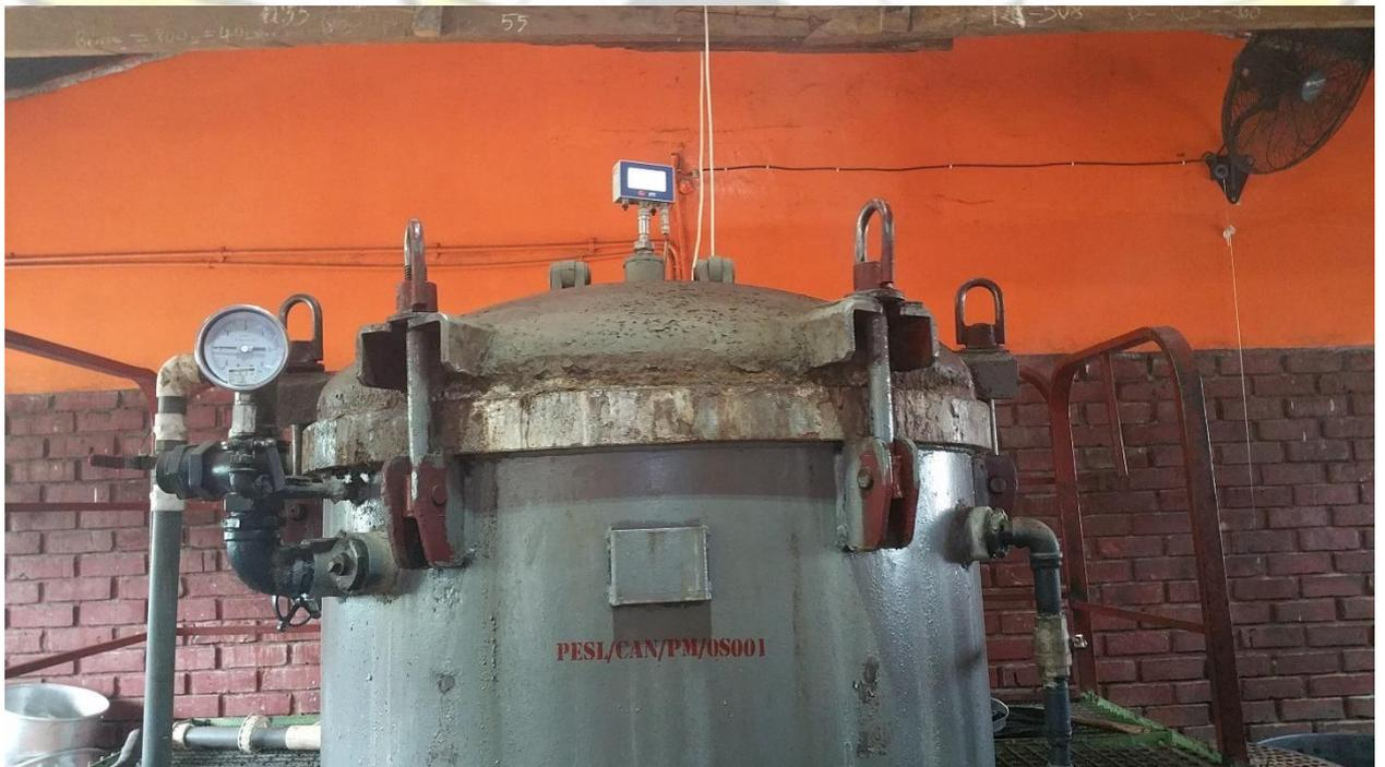
**Plate 14: A standing autoclave(retort) used by the company for sterilization (retorting)**
