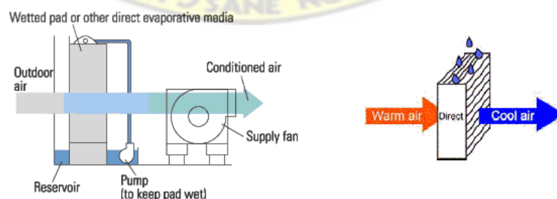
Figure 2.2 Diagram illustrating direct evaporative cooling (Bhatia, 2012)
