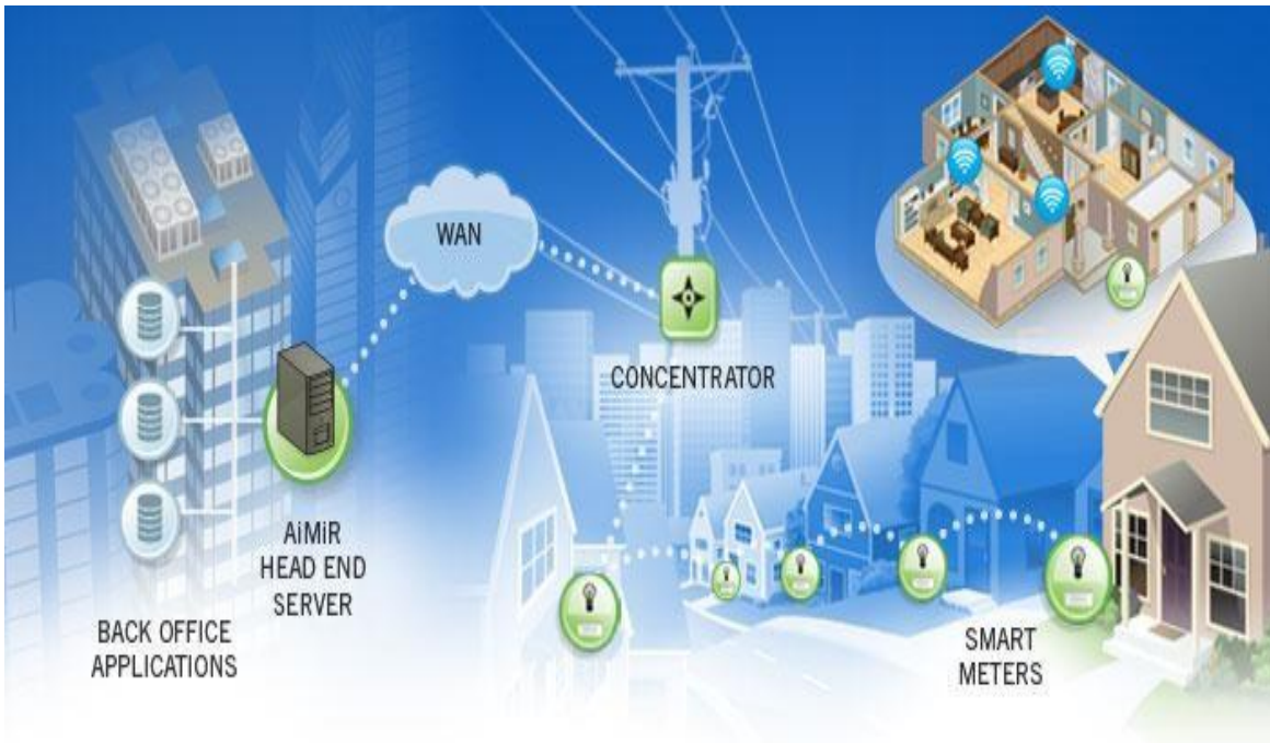
Figure 2-4 AMI solution architecture
