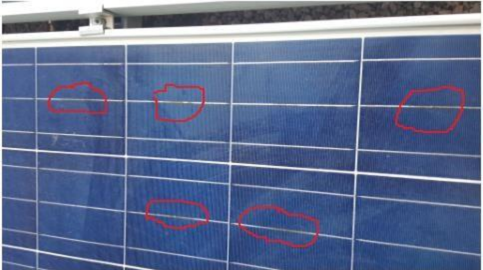
Snail crack propagating on module
