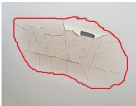
Back sheet delamination leading to cracks
