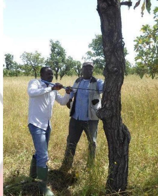
**Picture 3. 2 Techniques of extraction of measurement in the field. (CHABI, 2014) wood sample using increment borer. (CHABI, 2014)**
