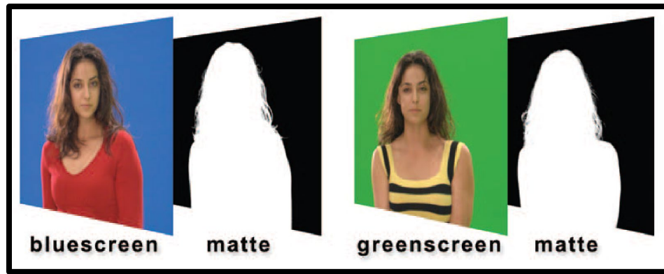
Plate 2. 9: Sample image of characters on blue and green screen and a matte ready for compositing
