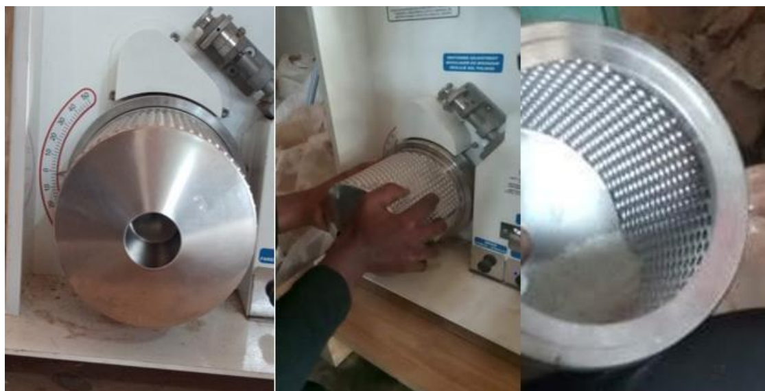
Plate 3.7: The section of the Zaccaria PAZ-1/DTA Lab rice mill for grading
