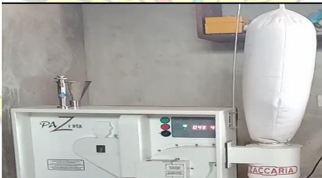
Plate 3.5: The section of the Zaccaria PAZ-1/DTA Lab rice mill for dehusking
