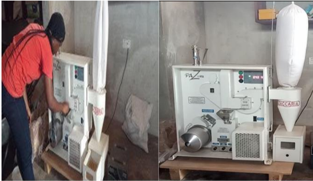
Plate 3.4: Milling of dried sample with Zaccaria PAZ-1/DTA Lab rice mill
