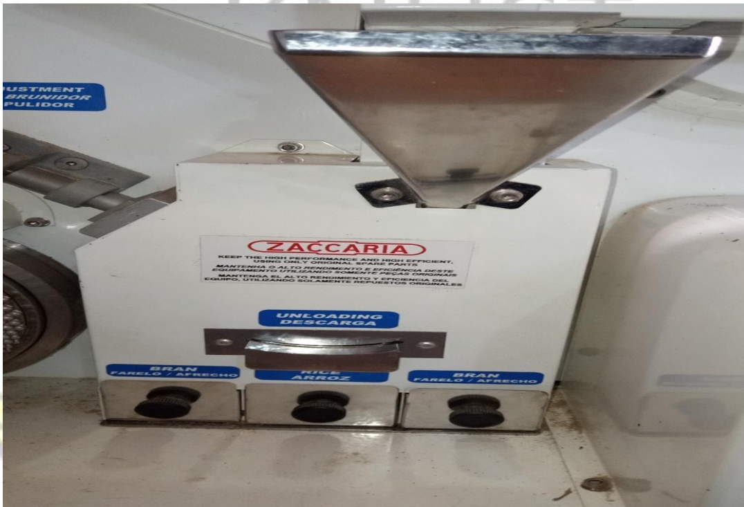
Plate 3.6: The section of the Zaccaria PAZ-1/DTA Lab rice mill for polishing / debraning
