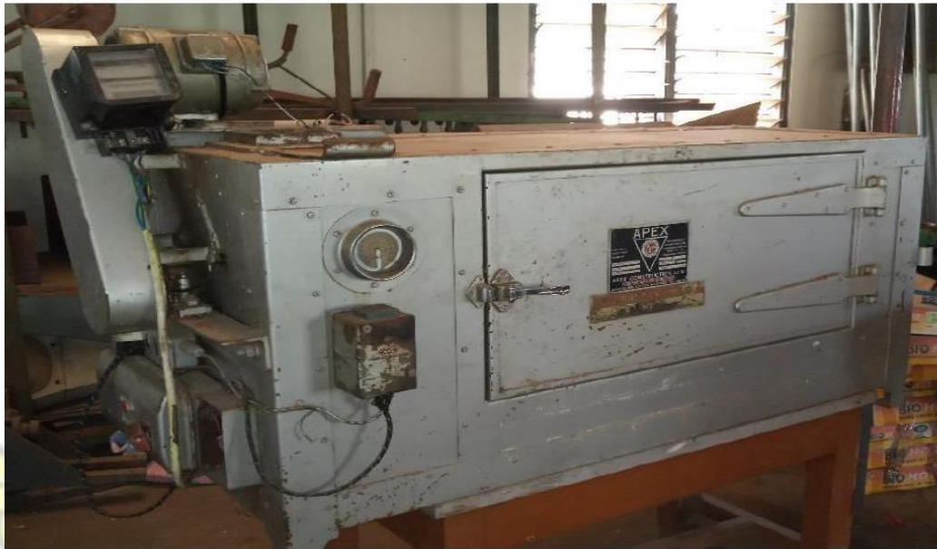
Plate 3.3: A fixed or static bed dryer
