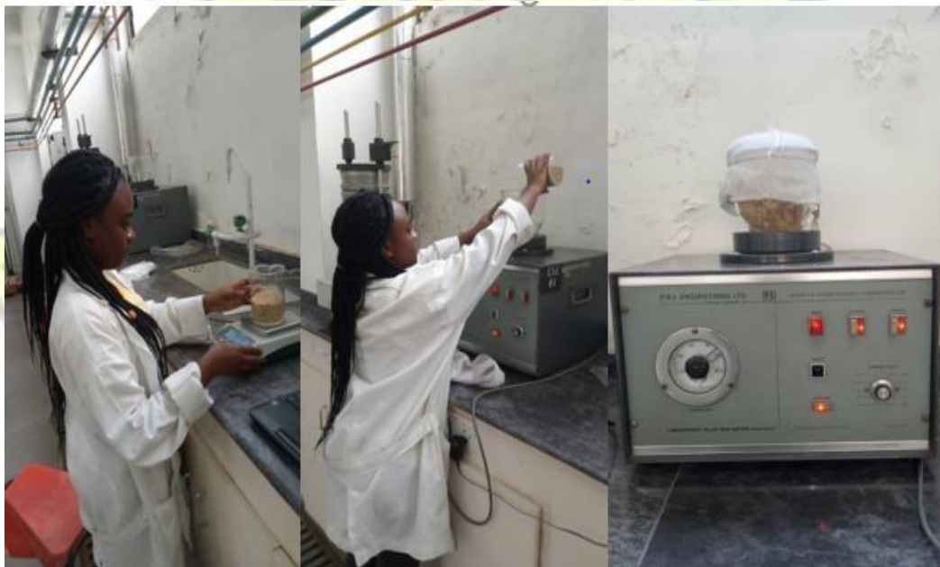
Plate 3.2: First stage drying of paddy using the fluidised bed dryer
