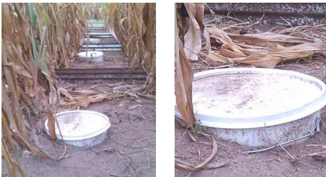
Plate 3.2 Chamber covered during emission study
