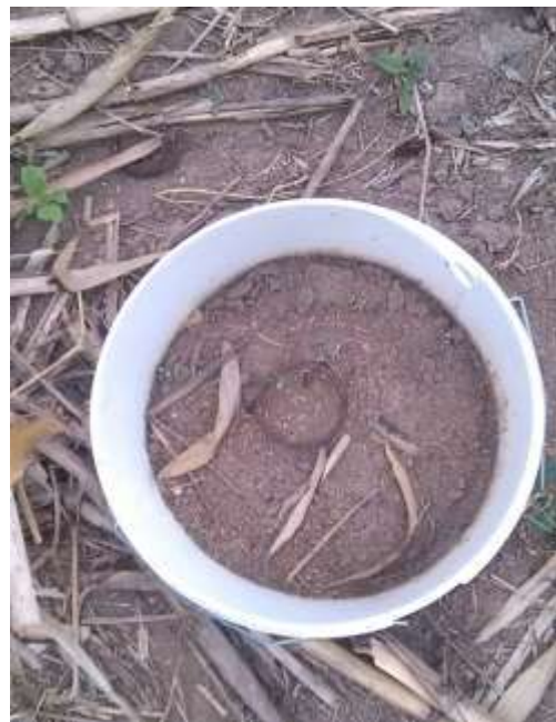
Plate 3.1 Chamber inserted in the soil before the emission study
