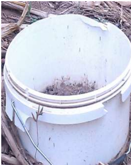
Plate 3.1 Chamber inserted in the soil before the emission study
