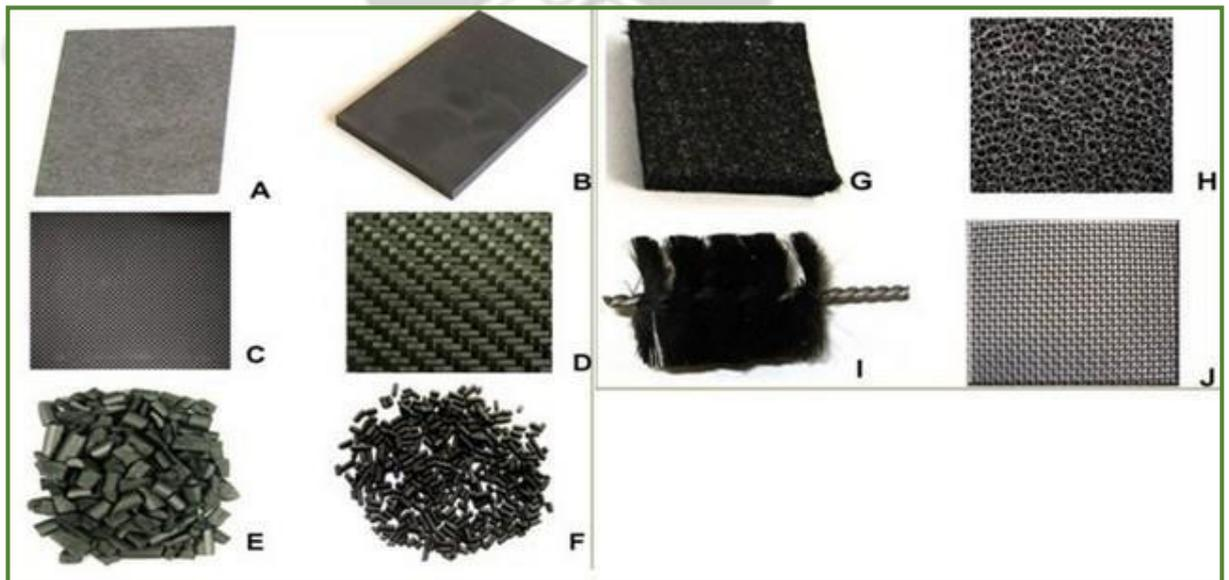
*Figure 2-9. Examples of electrode materials commonly used in MFCs [87] ( A-carbon paper, B-graphite plate, C-carbon cloth, D-carbon mesh, E-granular graphite, F-granular activated carbon, G-carbon felt, H-reticulated vitrified carbon, I-carbon brush, J-stainless steel mesh)*
