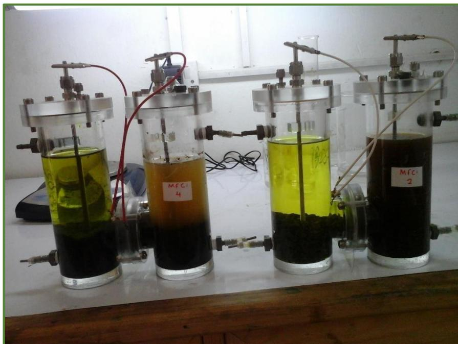
*Figure 3-2. The H-shaped Double chambered MFCs used in the study 3.2.2*
