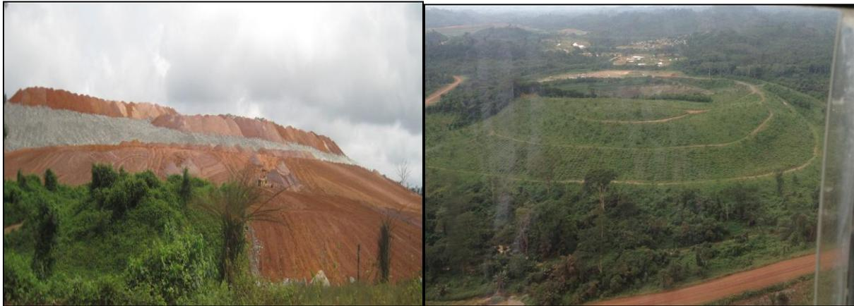
**Plate 1: View of encapsulation and aerial view after re-vegetation of the SE rock dump**
