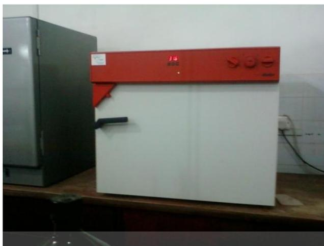
Figure 4.2: Electrical oven used in drying of the zeolite crystals
