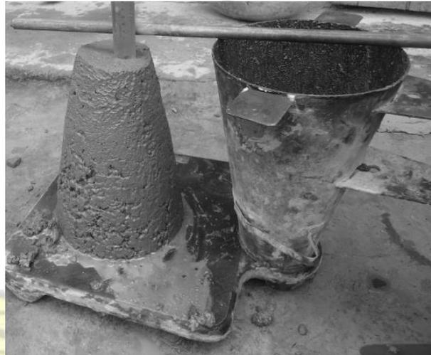
*Fig. 3.1 Slump test of PKS concrete*
