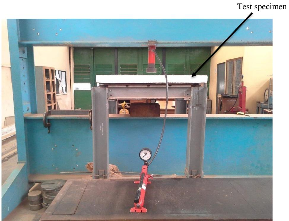
*Figure 3.12 Experimental set-up of loaded slabs*
