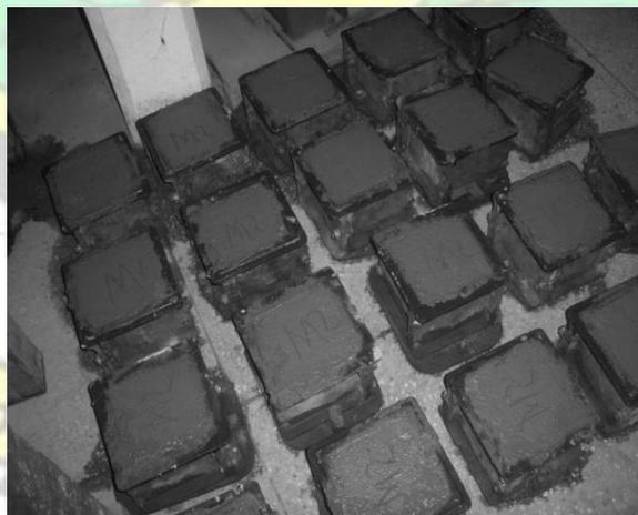
*Fig. 3.2 Sample of freshly cast concrete cubes*
