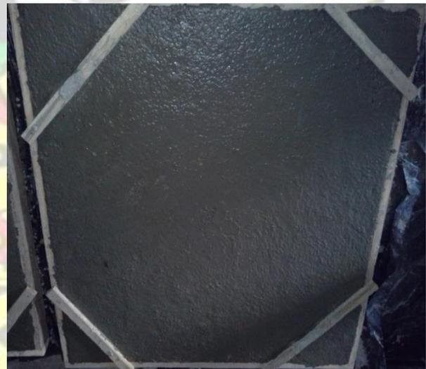
*Fig. 3.11 Sample of PKSC slabs*
