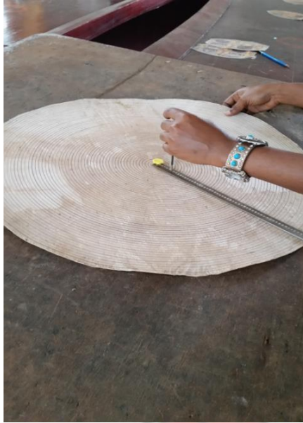
Plate 3.46: Marking the leather
