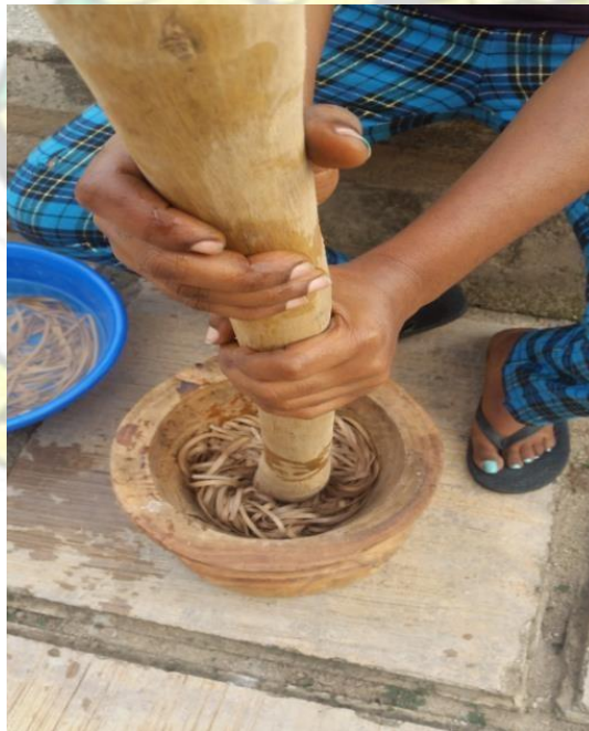
Plate 3.47: Pounding of leather strips
