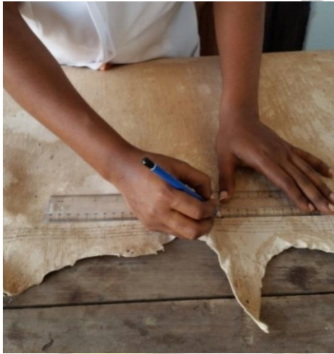
Plate 3.33: Marking out on the leather
