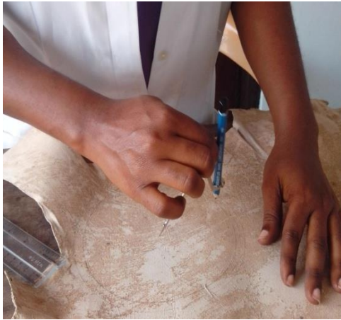
Plate 3.35: Marking out on the leather
