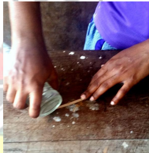
Plate 3.45: Burnishing the leather strip ii.
