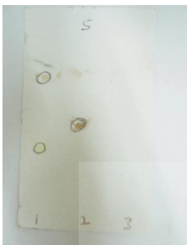
Figure 6.15: TLC chromatogram for DHA and Piperaquine phosphate pure samples compared with Arthemether mixed with Lumefantrine pure samples.
