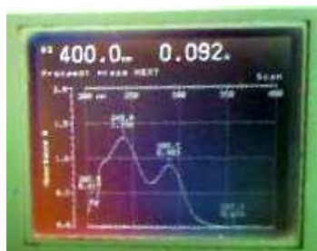
Figure 4.9: 5.00ml of 0.2%( w/v) dihydroartemisinin in methanol topped up to 50.00ml with 0.05M NaOH and heated at 50°C for 30minutes
