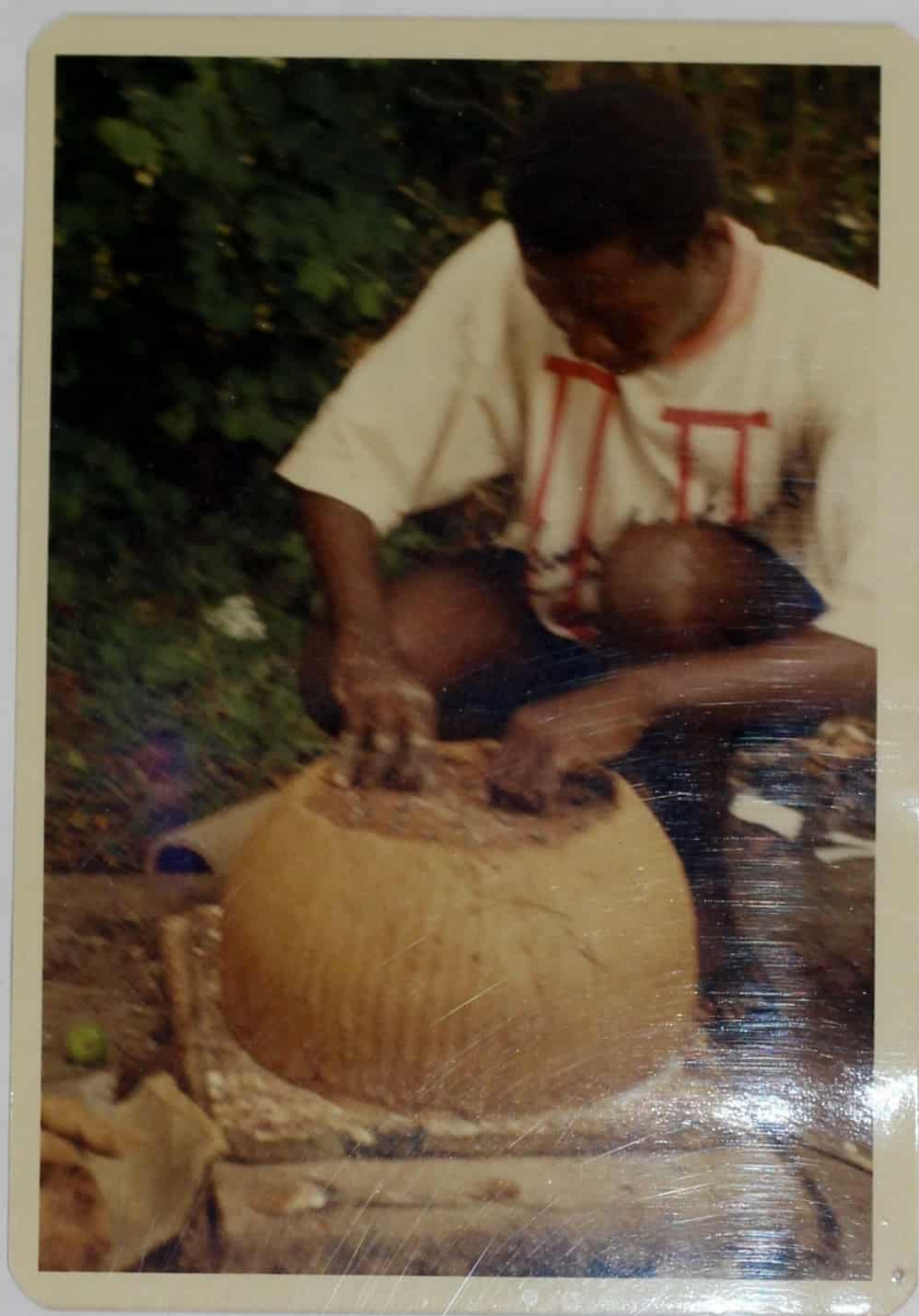
Plate 5. Fitting the metal grate in Oven.
