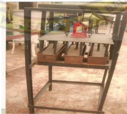
Figure 2.6.1 Briquette machine with bottle jack Source: (Ajobo, 2014)
