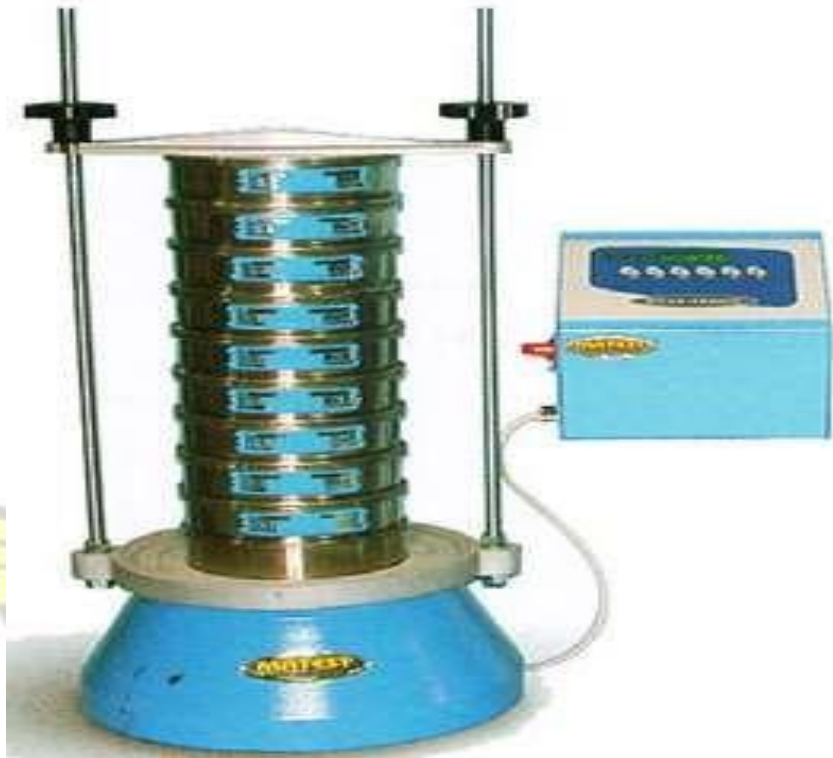
Figure 3.1: Sieves arranged in a stack with the mesh size increasing from bottom to top on mechanical shaker
