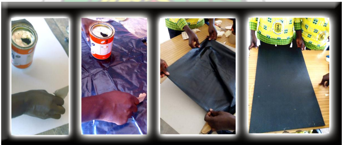
Plate 22: Covering the strawboard with lining material by gluing
