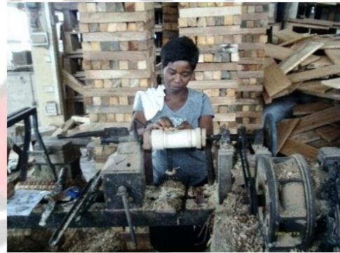
Plate 19. Sanding in lathing
