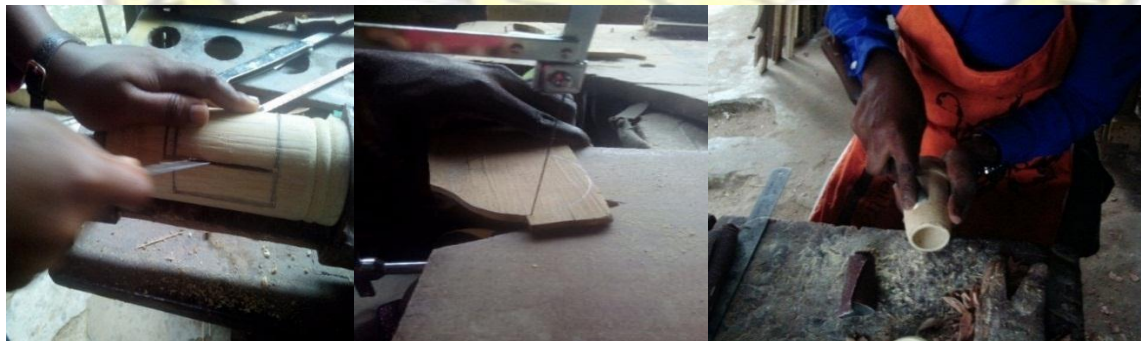
Plate 22. Creating and shaping openings for the containers
