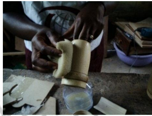
Plate 24. Application of sanding sealer
