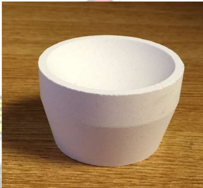
Figure 2.4: Cupel used for cupellation ( www.lmine.com )
