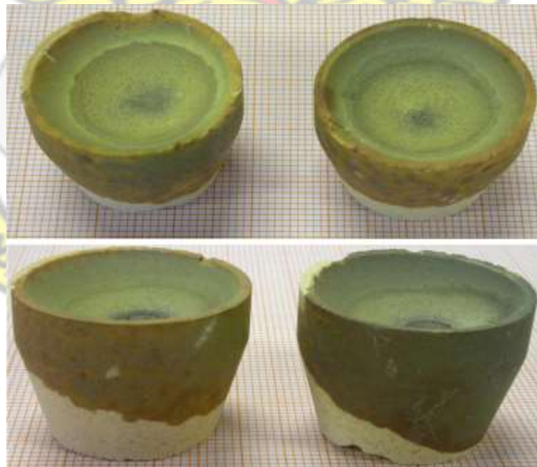
Figure 2.3: Cupels which have absorbed litharge during the cupellation (Battaini et al., 2014)
