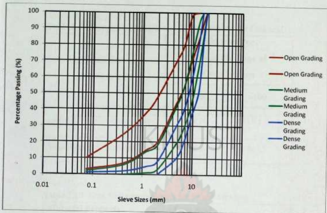
Figure 2.7: Open, medium and dense grading envelope for Otta seal (Overby and Pinard, 2007)
