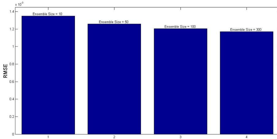
Figure 3.6: Plot of root mean square errors showing the effect of different ensemble size on the performance of ensemble Kalman filter
