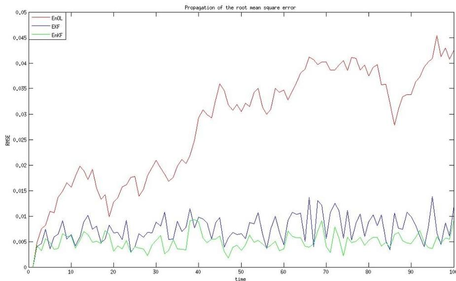
Figure 3.4: Plot of the root mean square error propagation by the different filters in the van der pol problem for the first experiment
