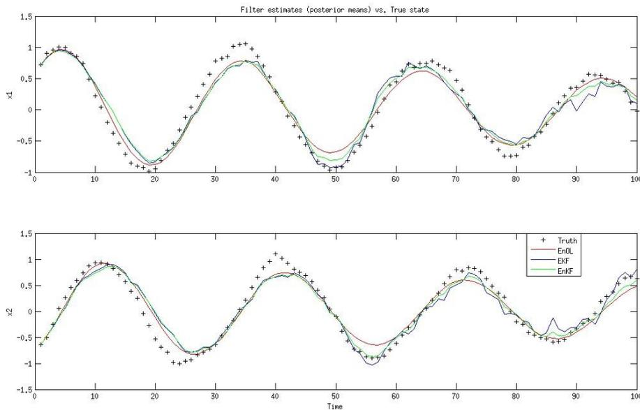
Figure 3.5: Plot of the state estimate from the different filters compared to the true state at  $R = I_2$
