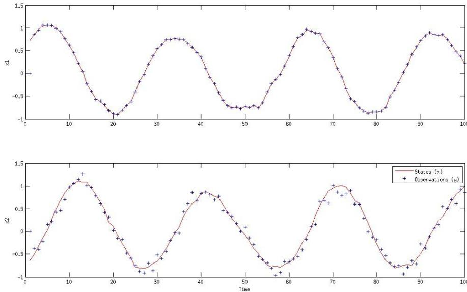
Figure 3.2: Plot of observation and truth generated in the van der pol problem for the first experiment
