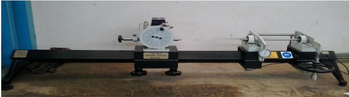
**Figure 3.5:** Tecquipment SMI MKII-torsion testing machine
