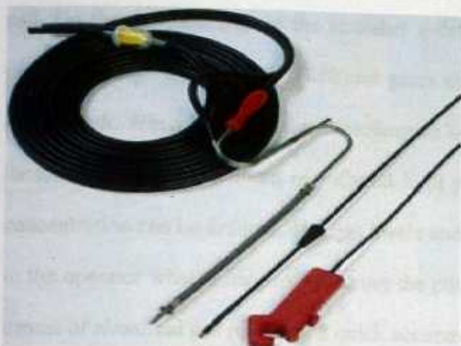
Figure 2.7: The metal hose and the metal sample probe of the OPUS 40 gas analyzer (Source: Opus 40 Analyzer manual)
