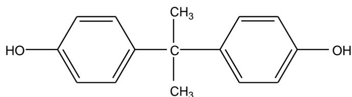
**Figure 1.1: Molecular structure of BPA**
