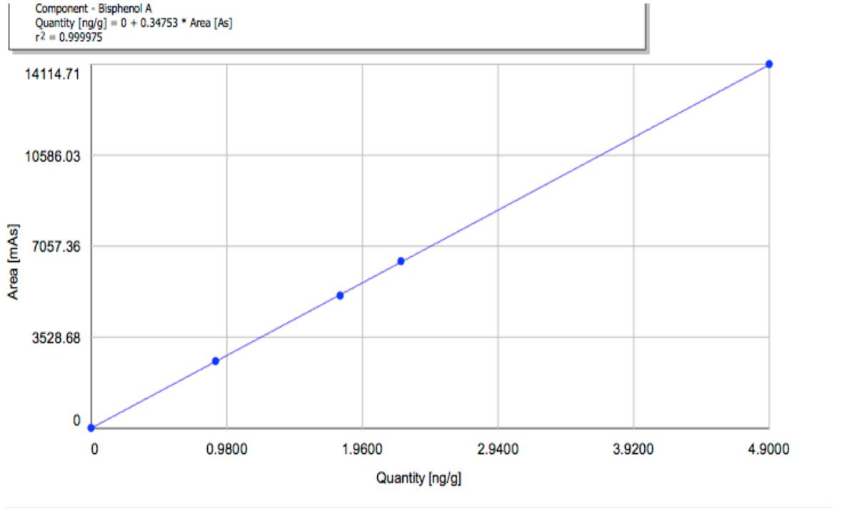
**Figure A1: Bisphenol A Concentration Calibration Curve**
