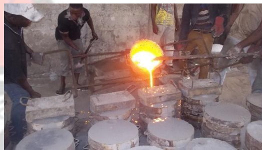
Figure B6 Mold Filling
