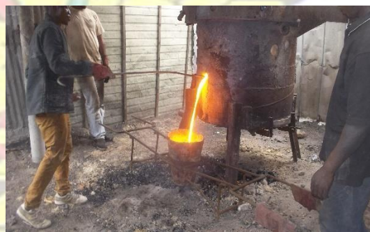
Figure B8 Tapping Melt.
