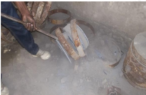
Figure B13 Breaking up Mold
