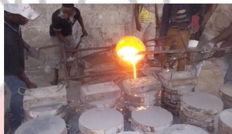
Figure.3.3. Pouring Melt into Mold
