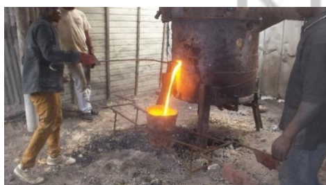
Figure.3.2. Tapping the Melt
