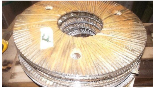
Figure 1.3. Mill Plate with Grooves. (Source: Kumasi Magazine, 2015)
