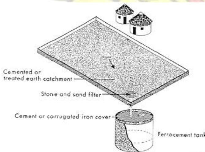
**Plate 2: Example of a ground catchment system**
