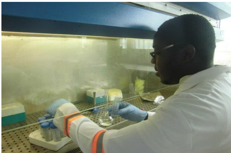
Plate 11: Addition of the acetonitrile to the mixture before vortex
