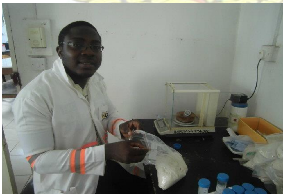
Plate 10: Weighing the samples and sodium chloride into the centrifuge tube
