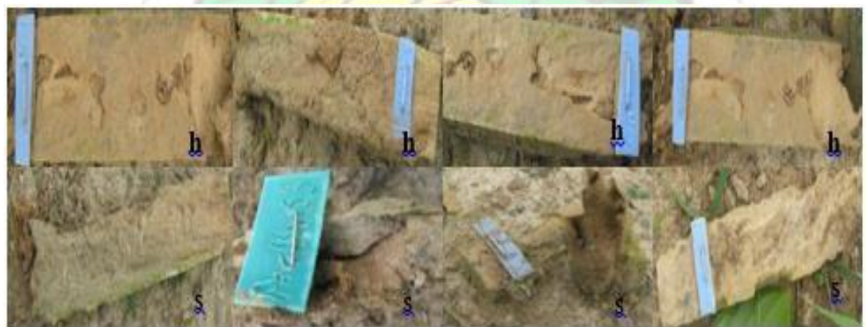
Plate 5.5: Failed heartwood (h) and sapwood (s) of A. robusta branch by the 16 th week of exposure.
