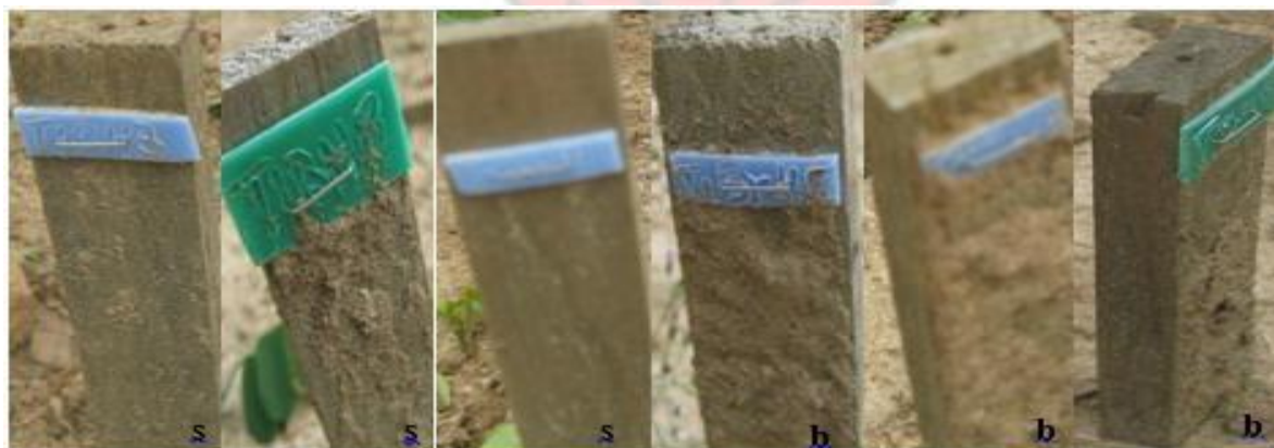
Plate 5.1: Stem (s) and branch (b) heartwoods of T. ivorensis during 16 th week of exposure
