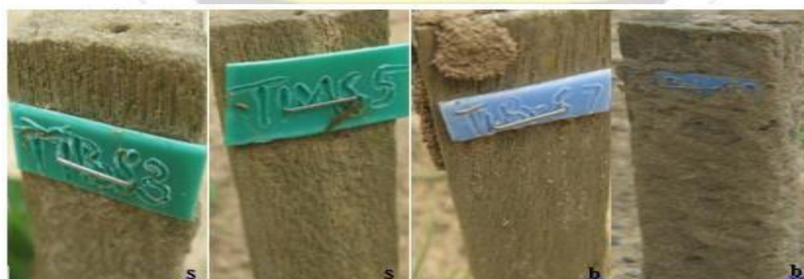
Plate 5.2: Stem (s) and branch (b) sapwoods of T. ivorensis during 16 th week of exposure.
