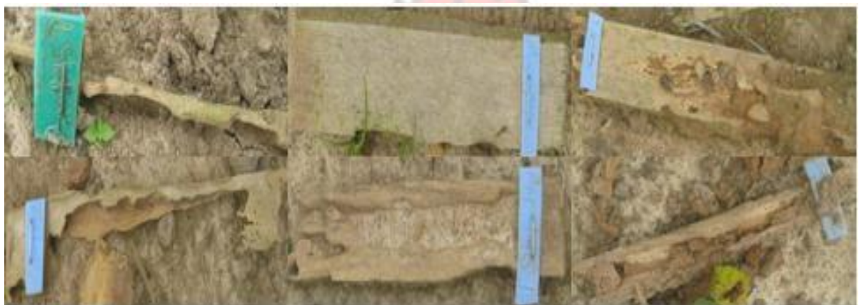
Plate 5.4: Failed sapwood stakes of A. robusta stem by the 16 th week of exposure
