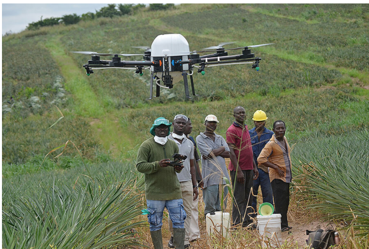
Figure 37: Drone spraying on pineapple farms at Adeiso, Ghana
