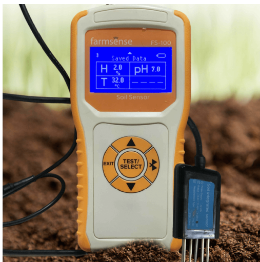
Figure 36: Soil tester produced by Sessi Technologies in Ghana.
