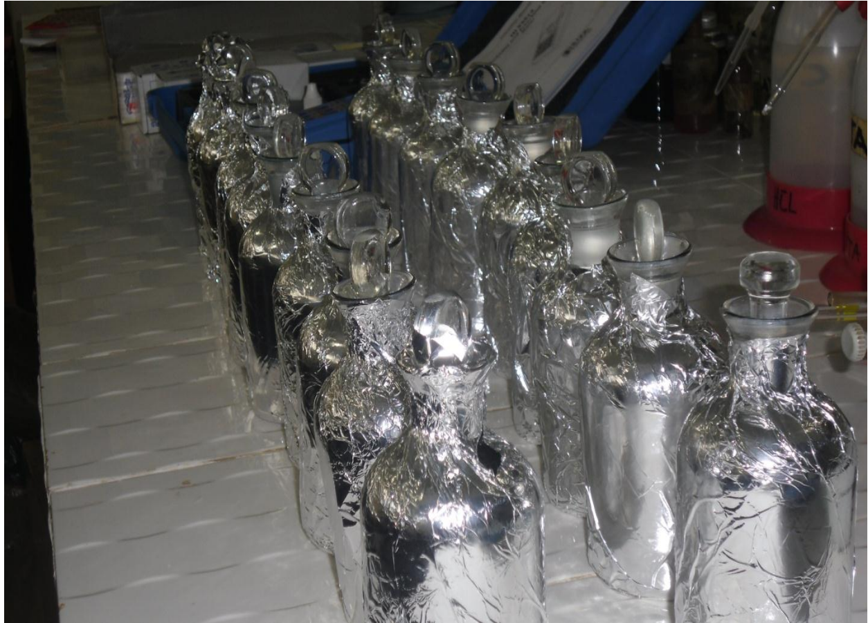
Plate 3. 1 Bottle test used for bulk decay coefficient determination
