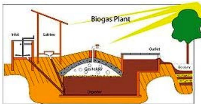
Figure 2.13 Typical layout of biogas plant (Source: Wikipedia, 2008)
