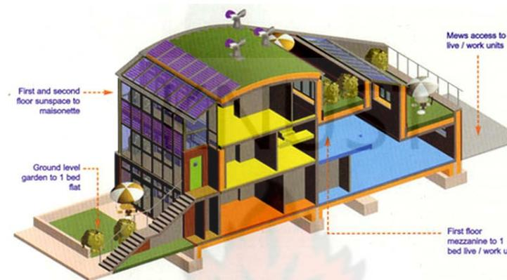
Figure 2.21 Isometric section through a typical BedZED building. (Source: diagram adopted from BedZED Eco-Village 2008)
