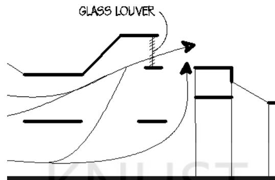
Figure 2.8 Operable elements provide natural ventilation.
