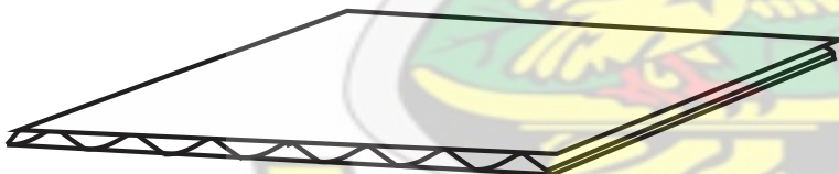
Figure 2.2: Double face corrugated board
