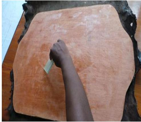
**Plate 24: Applying glue on the surface of the wooden board**
