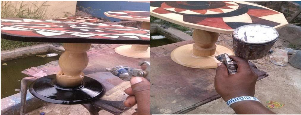
**Plate 42 A and B: Staining the Base of the Tables.**
