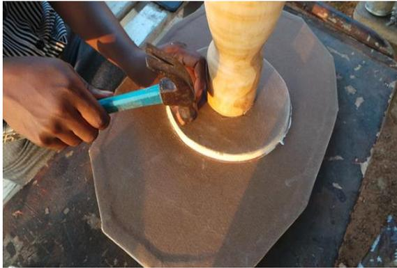
**Plate 38: Nailing the wooden stand to the board**
