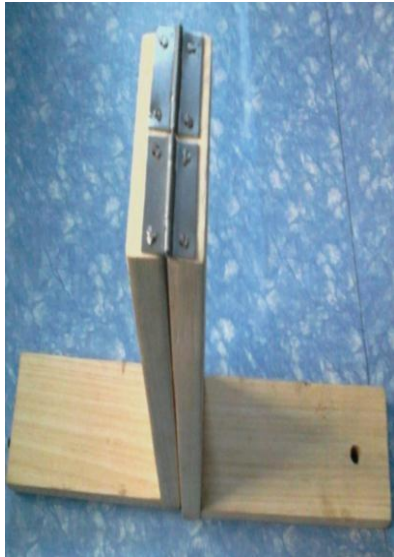
Plate 3.34: L-shapes joined with hinges
