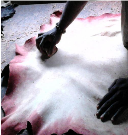
Plate 3.14: Sanding a sheet of leather
