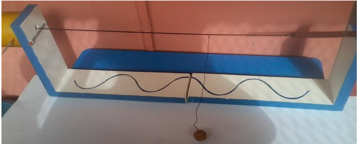
Plate 3.37: Developed “SES Demonstrator” for teaching “Wave” with weight attached
