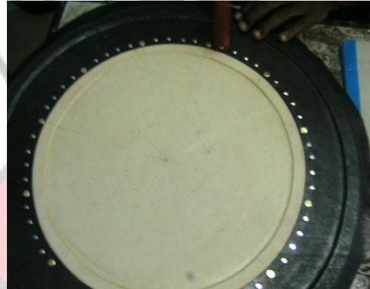
Plate 3.17: Divisions for numbering on the clock surface
