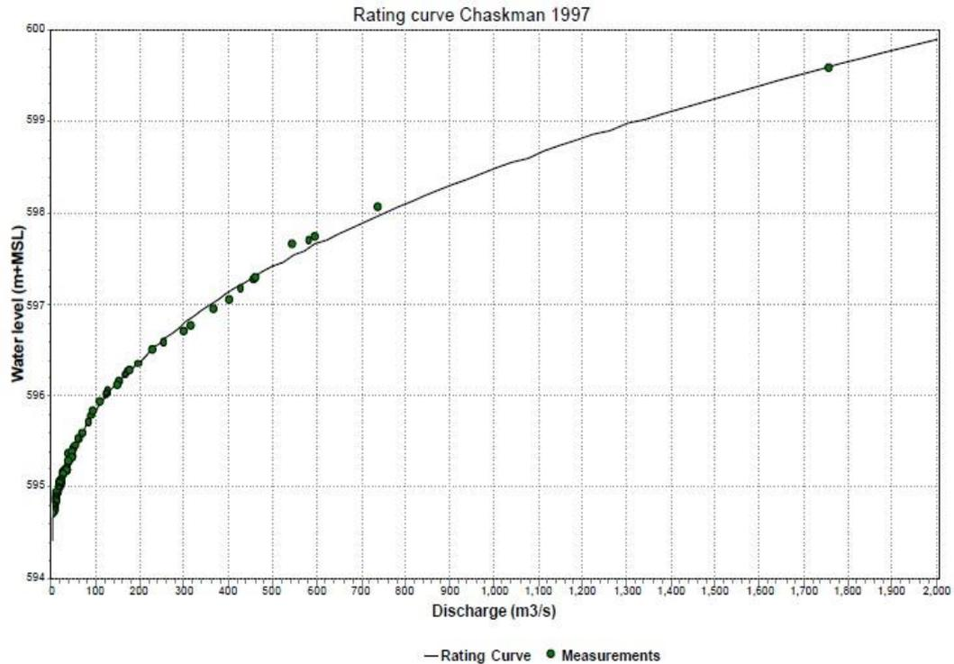
Figure 2.3 Stage discharge rating curve. (Hydrology Project Technical Assistance, 1999).
