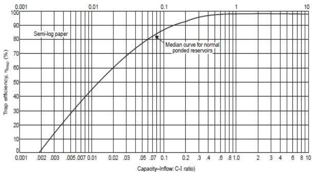
Figure 2.2 Trap efficiency curve for estimating sediment trapping in a conventional impounding reservoir (Brune, 1953).
