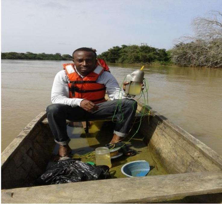
Plate 4.2 Suspended sediment sampling with the depth-integrating sampler
