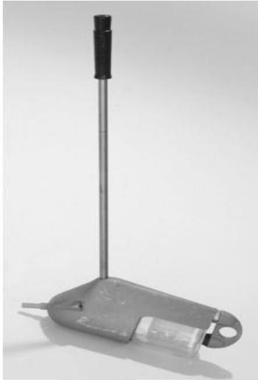
Plate 2.1 Depth Integration sampler.
