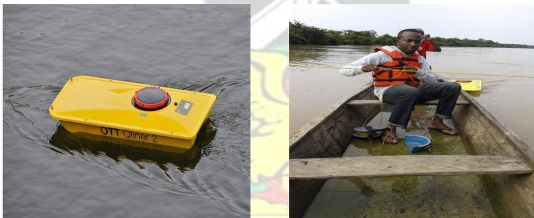
Plate 4.1 Discharge measurement with Qliner
