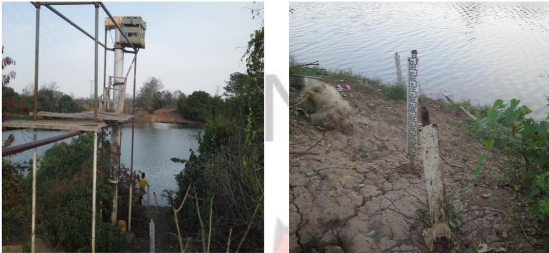
Plate 3.4 Automatic Gauge recorder and Staff Gauges at Chache gauged station
