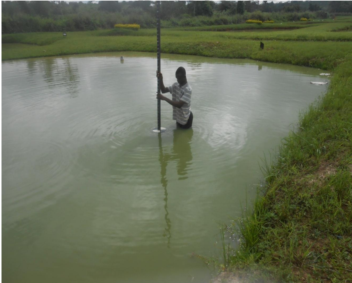
Plate 3: Measurement of pond transparency using Secchi disk
