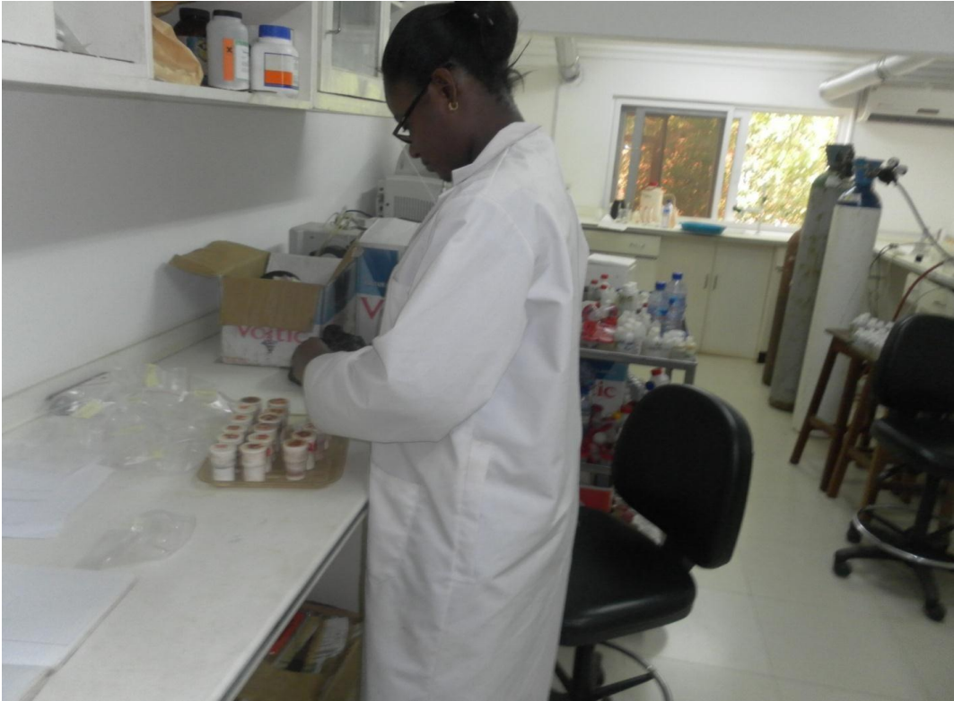
Plate 3.2: Extraction of PM 10 loaded filter paper in the laboratory
