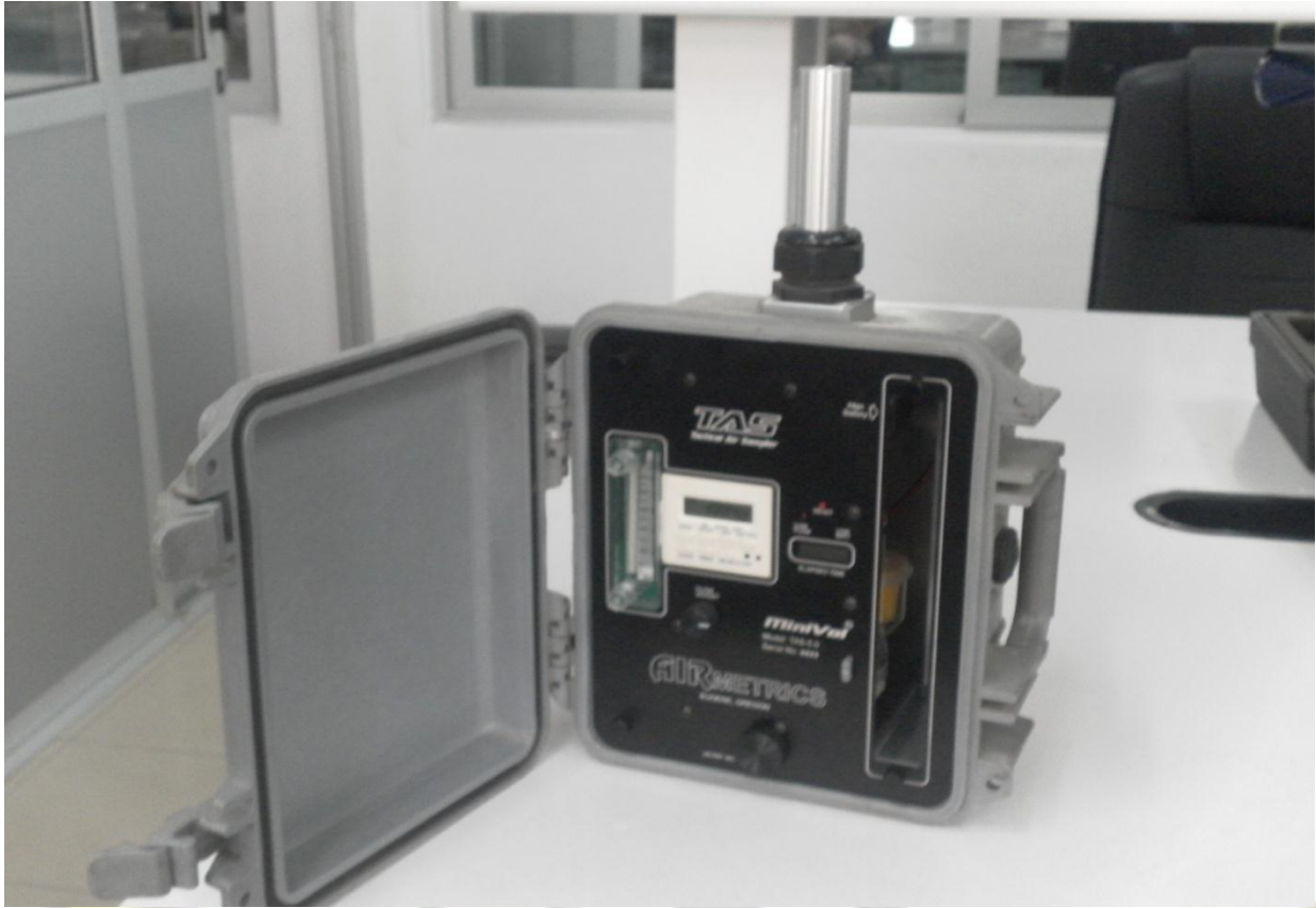
Plate 2.1: The MiniVol Air Sampler
