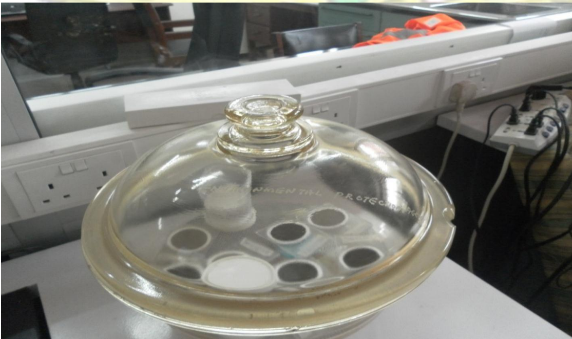
Plate 2: loaded quartz filter papers being conditioned in a desiccator.
