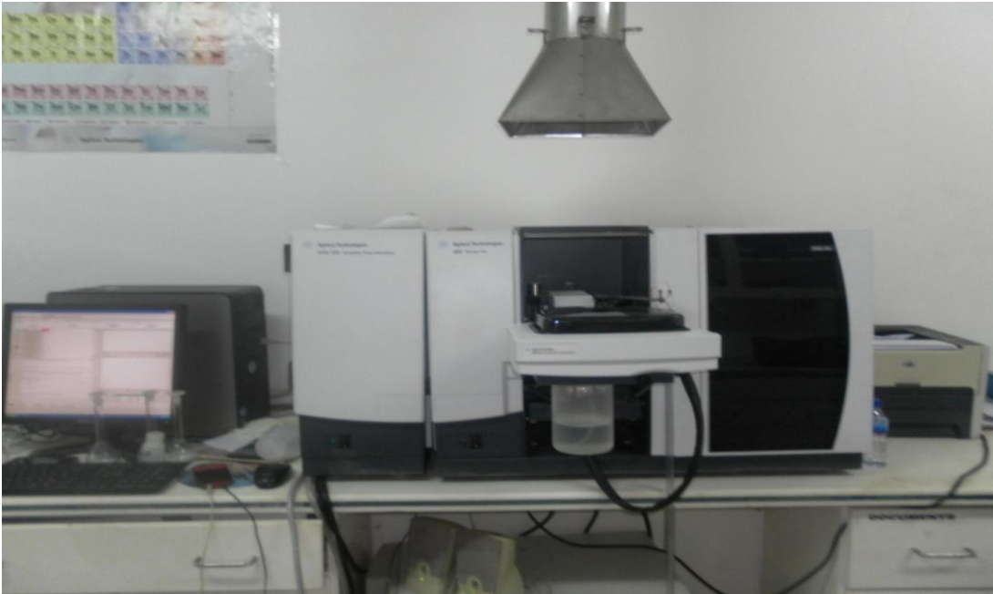
Plate 1: Atomic Absorption Spectrophotometer (model AA-200 Series; Agilent Technologies)
