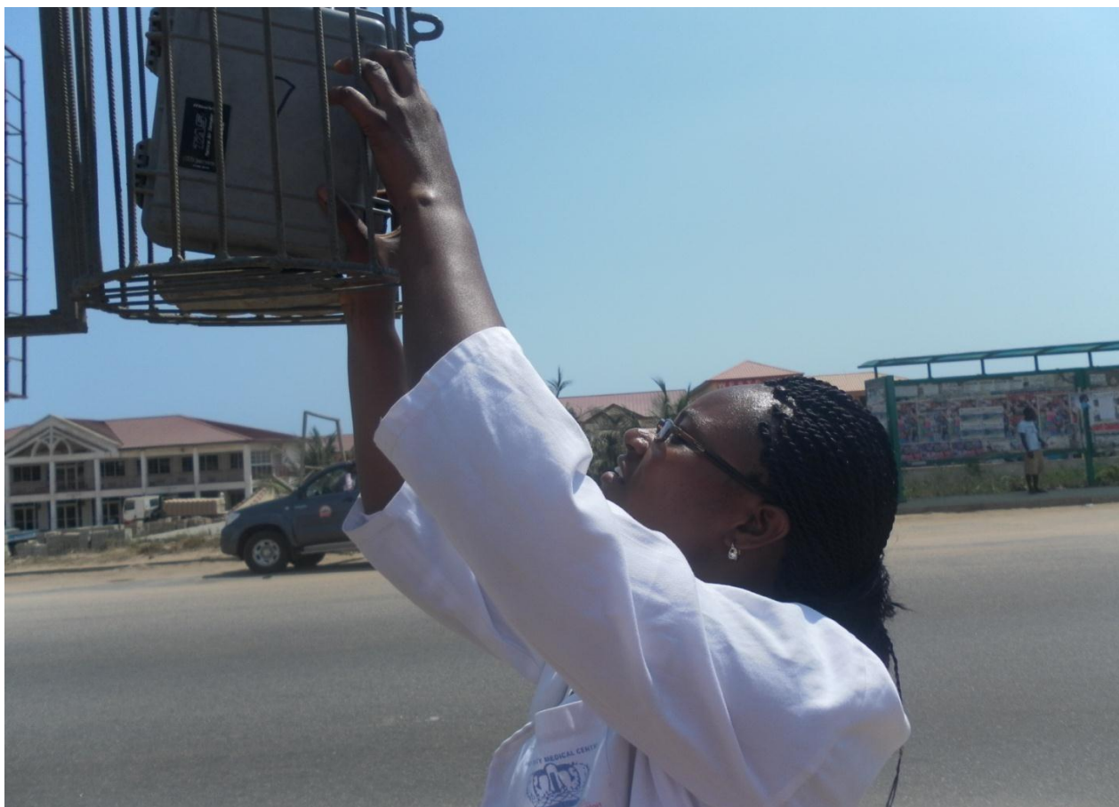
Plate 3.1: Mounting the Mini Vol.air samples at Weija.
